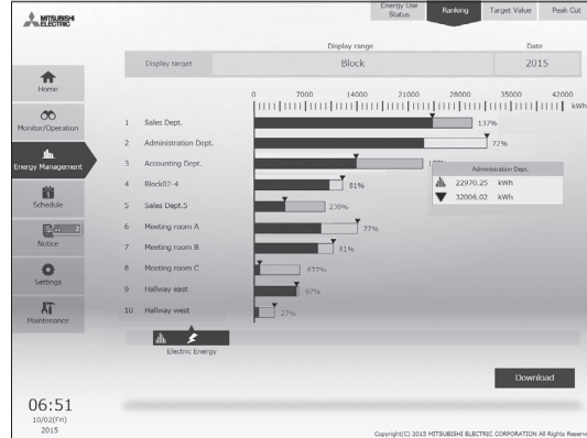
Energy Management Monitor (Ranking)
