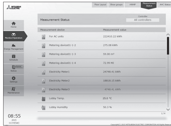
Measurement Status Monitor (Temperature Sensor/Humidity Sensor /Measurement Meter)
