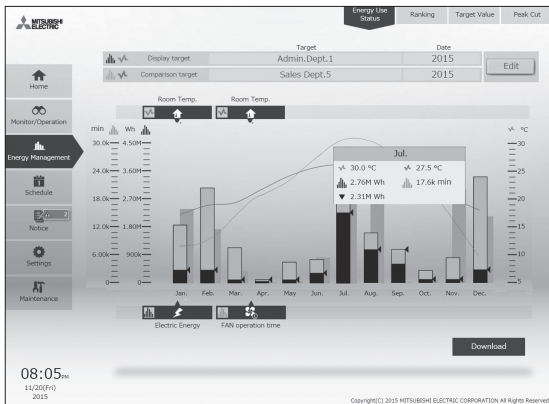
Energy Management Monitor (Energy Use Status)
