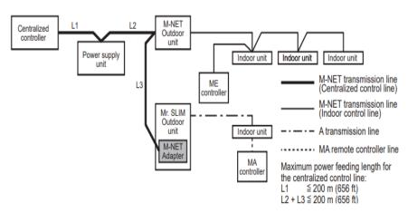
M-Net Interfaces are connected to indoor unit control boards via 5-pin connector on CN105. Outdoor unit adaptors are powered by outdoor control board CNMNT and CNVMNT connectors. All adapters have A and B terminals for connection to 2 wire M-Net network and shield connected to S ground terminal. Only the unit supplying M-Net 30VDC power has the S terminal grounded with ground accessory wire. The A and B terminals are not polarity sensitive. Installation requires 16AWG 2
