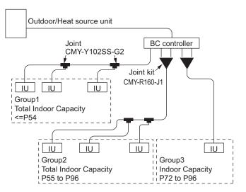
Fig.1. CMY-R160-J1 applying scheme
