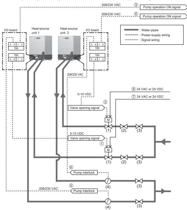
c) Schematic system diagram including heat-source units, water circuits, power supplies, and signals
