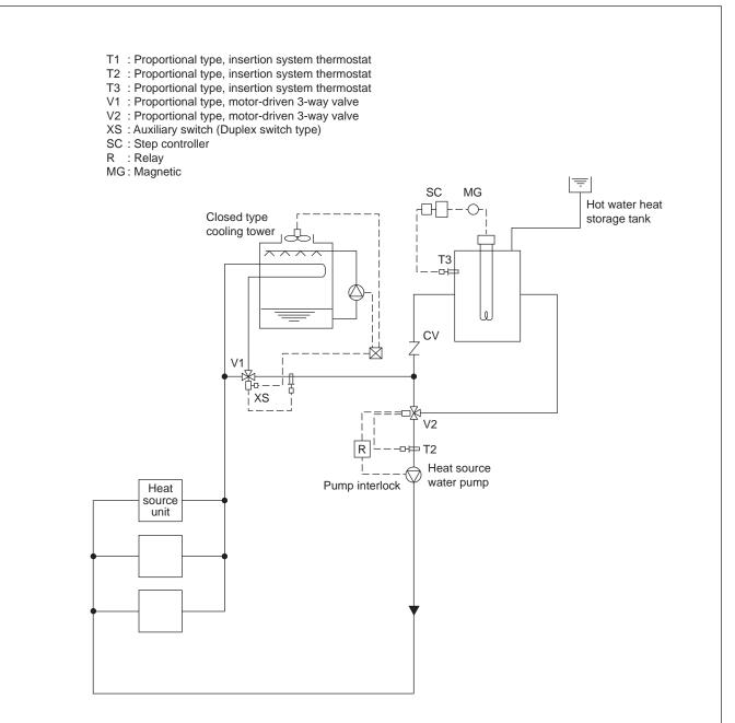
In the summer, as the circulation water temperature rises exceeding the set temperature of T1, the bypass port of V1 will open to lower the circulation water temperature. In the winter, if the circulation water temperature stays below 25°C [77°F], V2 will open/close by the command of T2 to keep the circulation water temperature constant.
