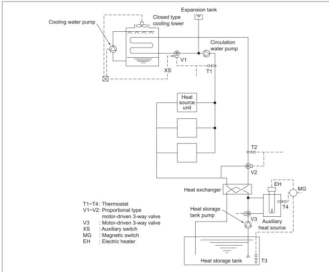
By detecting the circulation water temperature of the water heat source CITY MULTI system with T1 (around  $32^{\circ}$ C [90°F]) and T2 (around 20°C [68°F]), the temperature will be controlled by opening/closing V1 in the summer and V2 in the winter.
