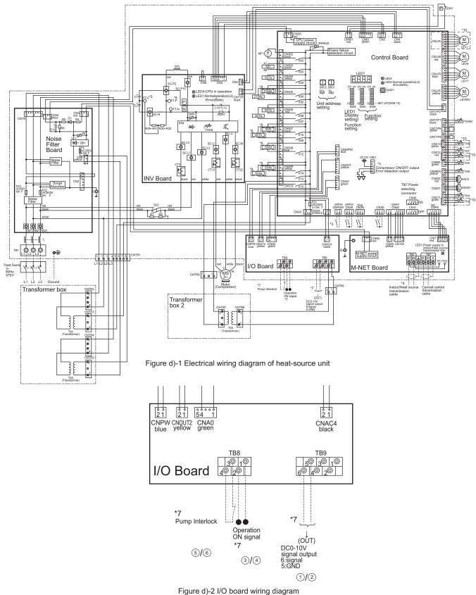
Figure d)-2 i/O board wiring diagra
