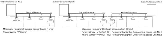
Fig. 1-1 The maximum refrigerant leakage concentration
