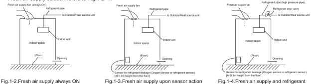
Fig.1-4.Fresh air supply and refrigerant shut-off upon sensor action
