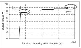
Figure b)-1 Analog signal output (when Dip SW4 (810) is set to OFF)
