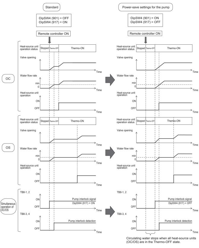
Power required by the pump is reduced compared to the standard settings.
