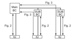
$^{\star}$ 7. When the piping length or the vertical separation exceeds the limit specified in Fig. 2, connect a sub BC to the system.
