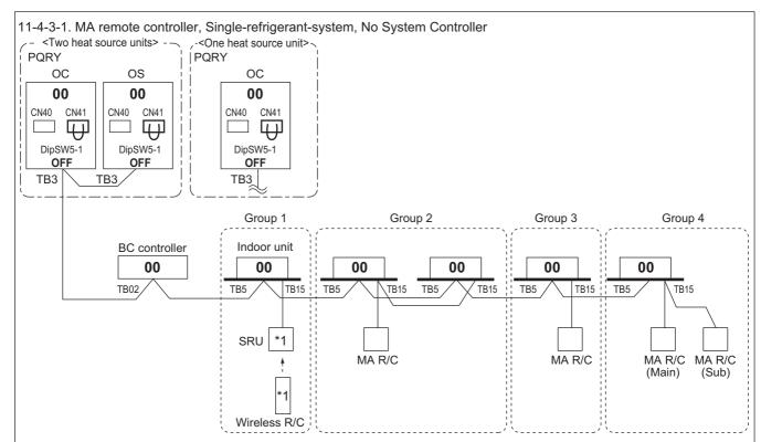
\*1 For Wireless R/C and Signal receiver unit (SRU), channel 1, 2 and 3 are selectable and should be set to same channel.
