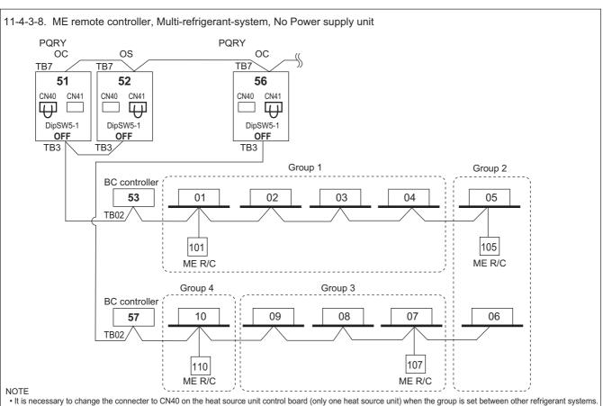
It is necessary to change the connecter to CN40 on the heat source unit control board (only one heat source unit) when the group is set between other refrigerant systems
