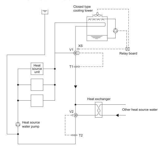
In the summer, as the inlet water temperature rises exceeding the set temperature of T1, the bypass port of V1 will close to lower the inlet water temperature. In the winter, if the inlet water temperature drops below 26°C [79°F], V2 will conduct water temperature control to keep the inlet water temperature constant.
