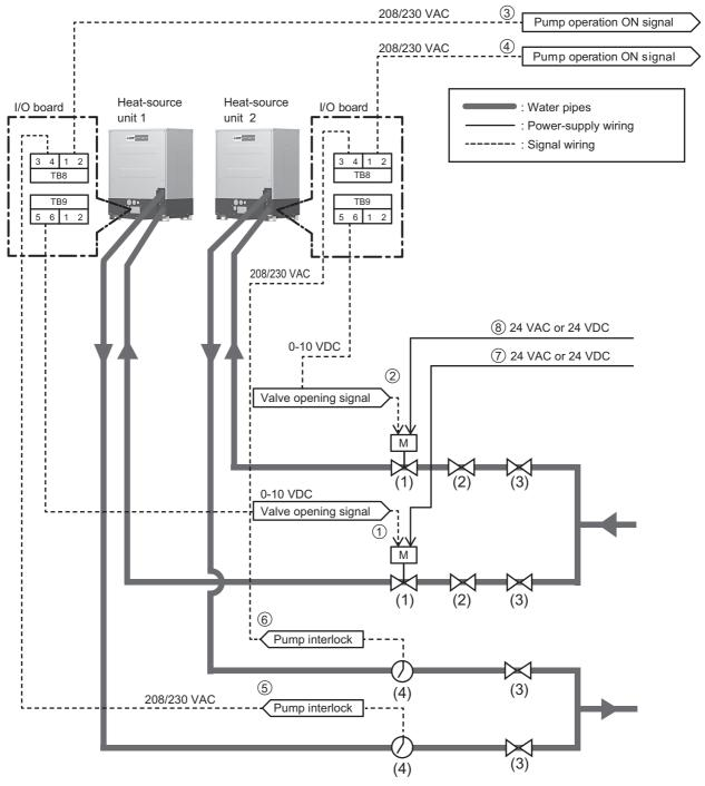
Figure c)-1 Schematic system diagram
