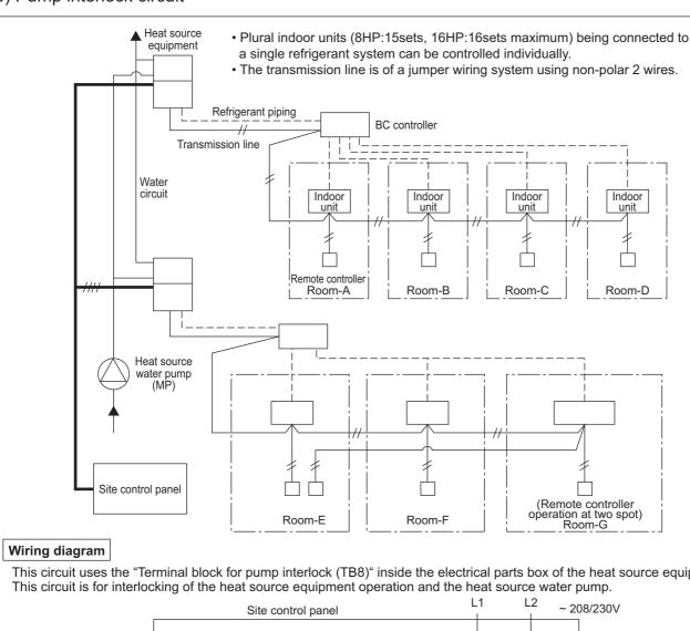
This circuit uses the "Terminal block for pump interlock (TB8)" inside the electrical parts box of the heat source equipment.
