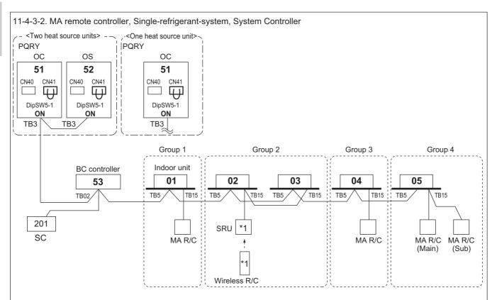
\*1 For Wireless R/C and Signal receiver unit (SRU), channel 1, 2 and 3 are selectable and should be set to same channel.
