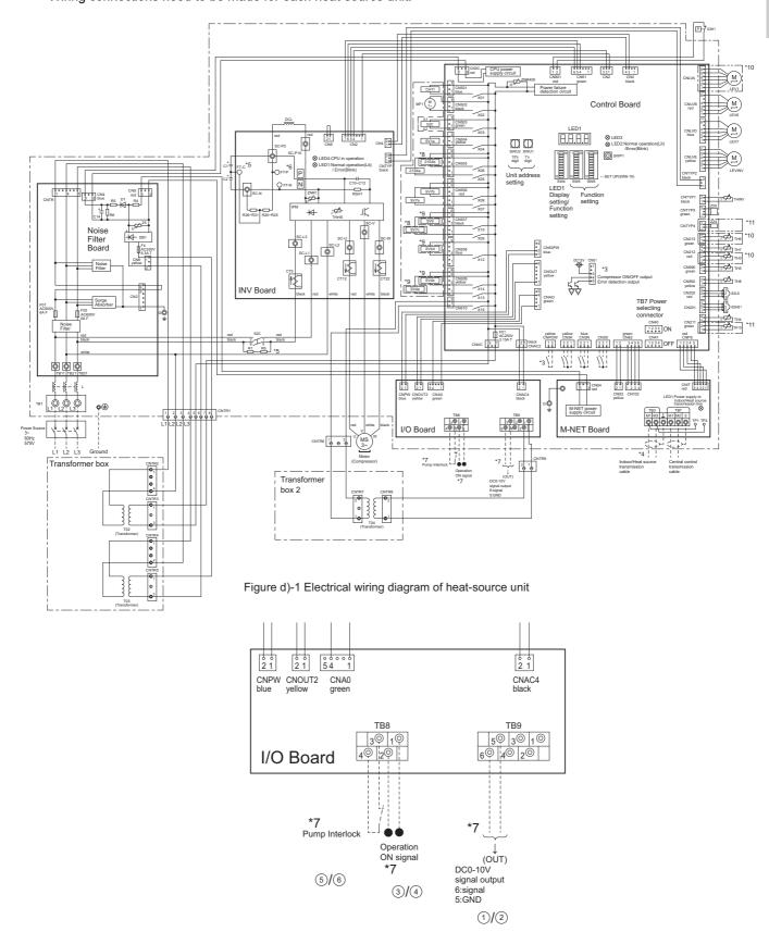
Figure d)-2 I/O board wiring diagram
