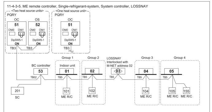
\*SC can be connected to TB3 side or TB7 side;
