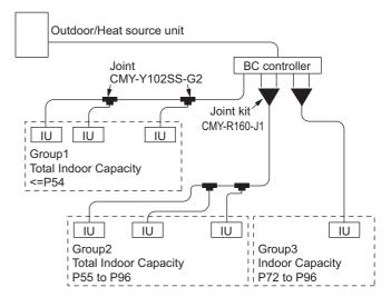
Fig.1. CMY-R160-J1 applying scheme
