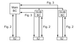
\*7. When the piping length or the vertical separation exceeds the limit specified in Fig. 2, connect a sub BC to the system.
