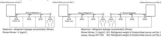
Fig. 1-1 The maximum refrigerant leakage concentration
