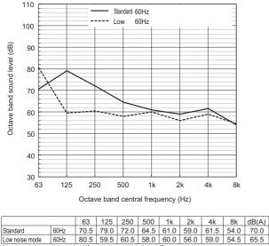
When Low noise mode is set, the A/C system's capacity is limited. The system could return to normal operation from Low noise mode automatically in the case that the operation condition is severe.
