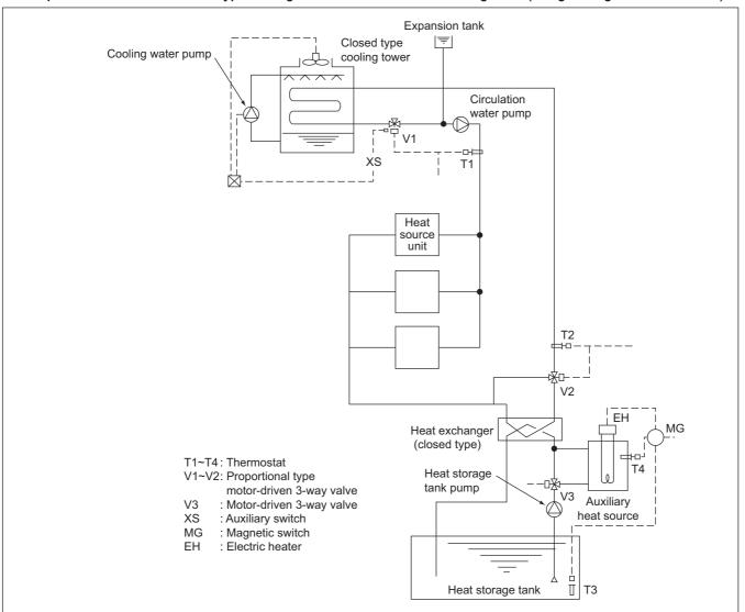
By detecting the inlet water temperature of the water heat source CITY MULTI system with T1 (around 30°C [86°F]) and T2 (around 20°C [68°F]), the temperature will be controlled by opening/closing V1 in the summer and V2 in the winter.
