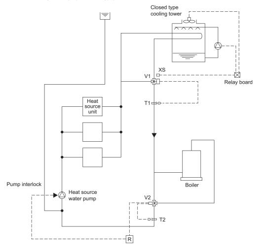
In the summer, as the inlet water temperature rises exceeding the set temperature of T1, the bypass port of V1 will close to lower the inlet water temperature. In the winter, if the inlet water temperature drops below 25°C [77°F], V2 will conduct water temperature control to keep the inlet water temperature constant.
