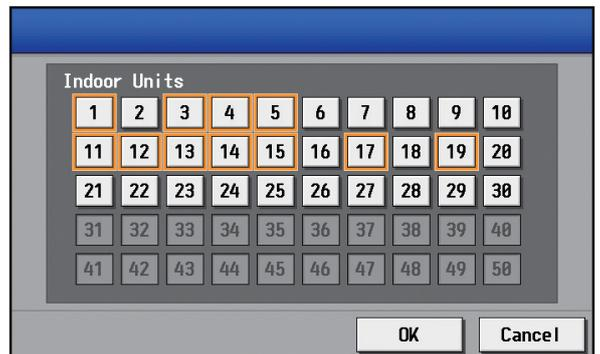
Note: Each LOSSNAY unit can be interlocked with up to 16 air conditioners.
