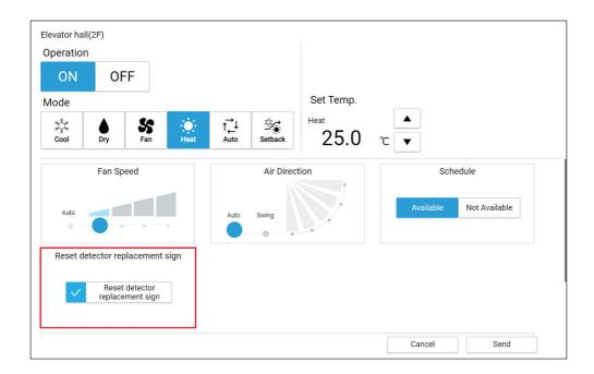
How to reset the detector replacement sign
