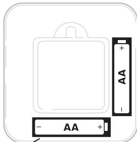
Insert fresh alkaline AA batteries and reinstall controller. Match the polarity of the batteries with the + / - marks inside the battery compartment.
