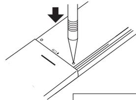
Press the Reset button with an object that has a narrow end.
