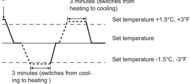
■ Because the room temperature is automatically adjusted in order to maintain a fixed effective temperature, cooling operation is performed a few degrees warmer and heating operation is performed a few degrees cooler than the set room temperature once the temperature is reached (automatic energy-saving operation).
