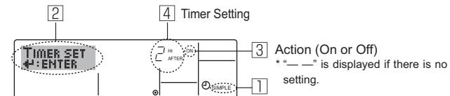
1. Be sure that you are at a standard control screen, and that the simple timer indicator is visible in the display (at ①). When something other than the Simple Timer is displayed, set it to SIMPLE TIMER using the function selection of remote controller (see 8.[4]–3 (3)) timer function setting.
