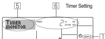
1. Be sure that the simple timer indicator is visible on the screen (at ①).
