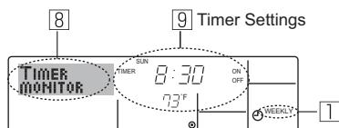
1. Be sure that the weekly timer indicator is visible on the screen (at ①).
