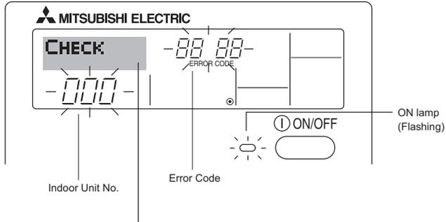
If you have entered contact number to be called in the event of a problem, the screen displays this number. (You can set this up under Function Selection of remote controller. For information, refer to section 8.)
