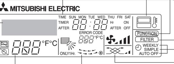
**Airflow up/down direction indicator**
