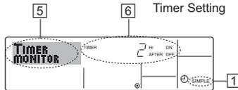
1. Be sure that the simple timer indicator is visible on the screen (at 1).
