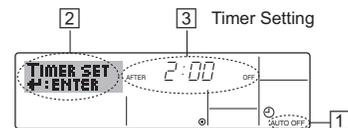
1. Be sure that you are at a standard control screen, and that the Auto Off timer indicator is visible in the display (at 1). When something other than the Auto Off Timer is displayed, set it to AUTO OFF TIMER using the function selection of remote controller (see 8.[4]-3 (3)) timer function setting.
