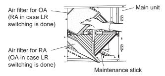
(3) Remove the back filters from the main unit with the maintenance stick.
