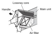
(3) After pulling out the Lossnay cores, remove filter guides, then remove the air filters, located at the bottom left and right of the Lossnay cores, as below.
