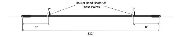
Heater is flexible and can be bended on the Field to Maximum 1" Round Radius
