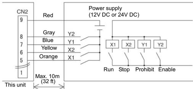
Use relays X1, X2, Y1, and Y2 that meet the following specifications.
