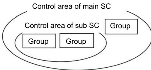
This system controller is designed as a main controller, so it cannot be controlled by a main SC (such as Gateway).
