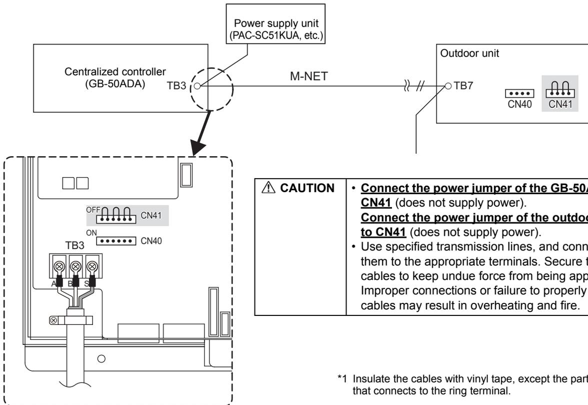
**CAUTION** • **Connect the power jumper of the GB-50ADA to CN41** (does not supply power). **Connect the power jumper of the outdoor unit to CN41** (does not supply power).
