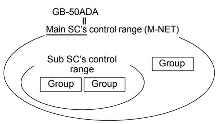
GB-50ADA is exclusively for use as a Main SC. It cannot be used as a Sub SC or controlled from a Main SC.
