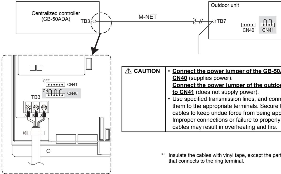
**CAUTION** • **Connect the power jumper of the GB-50ADA to CN40** (supplies power). **Connect the power jumper of the outdoor unit to CN41** (does not supply power).
