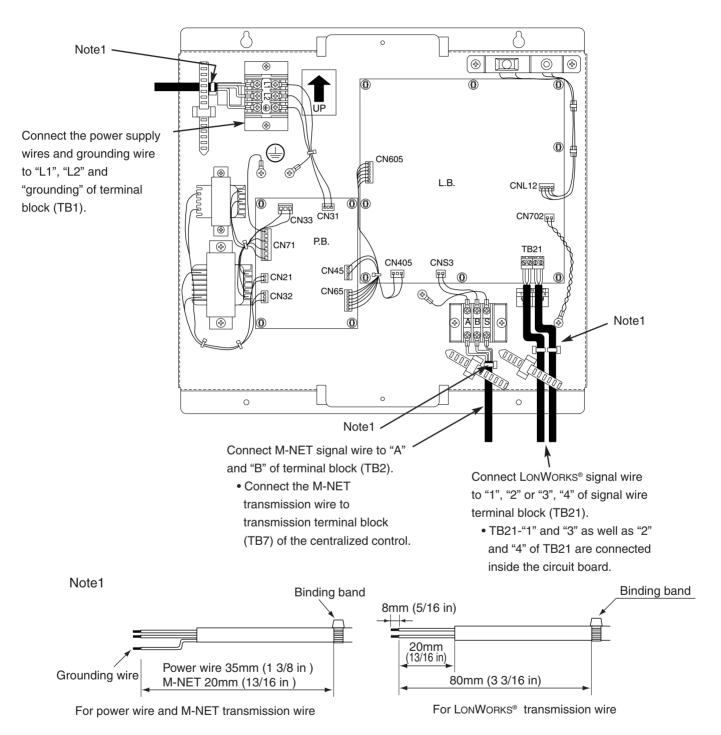
Attach the appended binding band to the power wire and transmission wire, and fasten it, positioning the area at inner side than the wire clamp.
