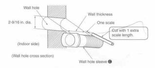
Be sure to use wall hole sleeve **()** to prevent the outdoor connecting wires from contacting with metal part in the wall and to prevent damage by rat in case the wall is hollow.
