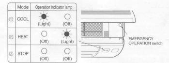
In starting the heating operation, indoor unit fan may not operate to prevent blowing cool air. Please wait for a few minutes until the temperature of heat exchanger rises and warm air blows out.
