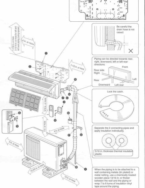
Units should be installed by licensed contractor according to local code requirement.
