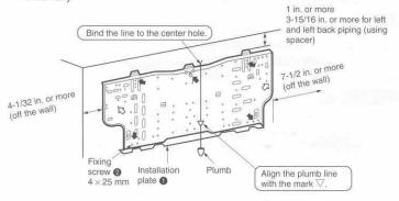
To prevent the installation plate from vibrating, be sure to fix the holes as indicated by the arrows  $\$  . Also, fix the holes as indicated by the arrows  $\$  as much as possible.
