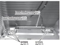
Pix the base heater (1) with the heater
