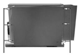
F. Using the screws provided, install the Front panel.
