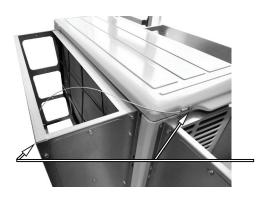
G. Install provided Lanyards to cabinet chassis with the existing screws as shown. Tighten the 2 screws already installed on the Front panel.
