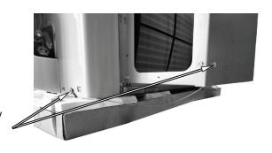
**NOTE:** Windblockers are used to protect the heat exchanger from direct wind exposure. Windscreens are required for operations where the ambient temperature is less than -5° Celsius.
