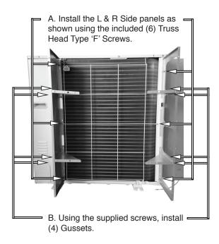
C. Install the Front panel using the provided screws onto the L & R Side panels and Gussets as shown.
