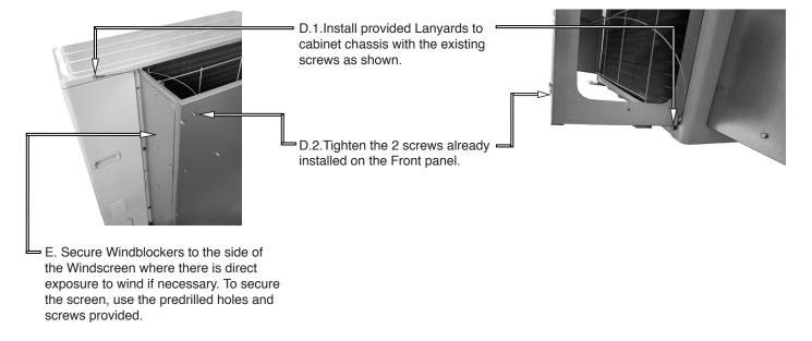
**NOTE:** Windblockers are used to protect the heat exchanger from direct wind exposure. Windscreens are required for operations where the ambient temperature is less than -5° Celsius.
