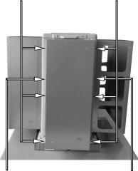
F. Secure windblocker(s) to the side of the windscreen where there is direct wind exposure if necessary. To secure the blocker to the windscreen, use the predrilled holes and four screws provided.
