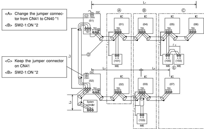
\*1: When the power supply unit is not connected to the transmission line for centralized control, disconnect the male power supply connector (CN41) from ONE outdoor unit in the system and connect it to CN40.
