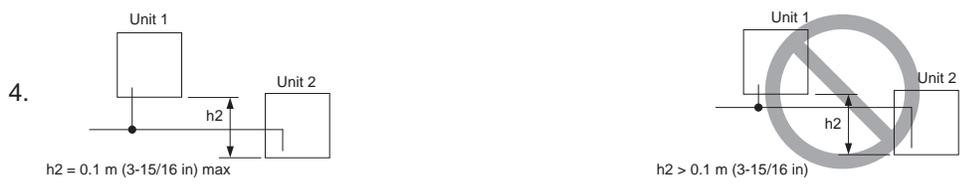
The NG example shows that oil accumulates into unit 2 while unit 1 is in operation, and unit 2 is stopped. Difference between unit and unit in height (h2) should be 0.1 m (3-15/16 in) or below.
