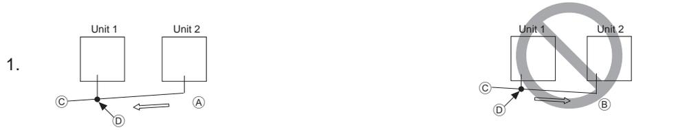
The NG example shows that oil accumulates because the units are installed on a reverse gradient while unit 1 is in operation, and unit 2 is stopped.
