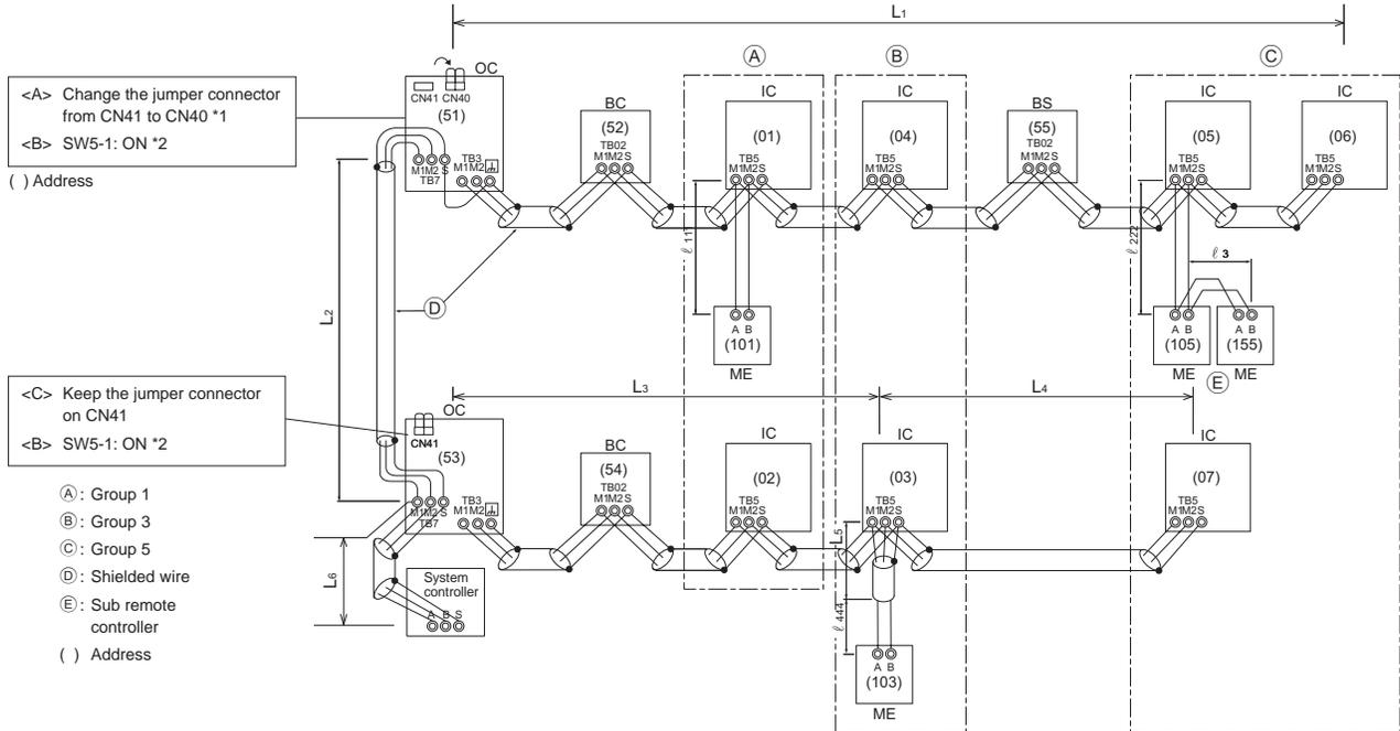
\*1: When the power supply unit is not connected to the transmission line for centralized control, disconnect the male power supply connector (CN41) from ONE outdoor unit in the system and connect it to CN40 (except TKMU model). When the System controller is connected to TB7 side and TKMU outdoor unit model is used, connect a PAC-SC51KUA to TB7 side. If a PAC-SC51KUA cannot be used, connect the System controller to TB3 side. Up to three System controllers can be connected to TB3 side.
