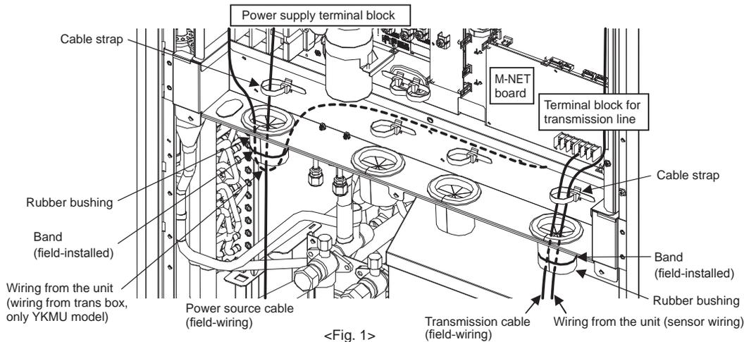
Note 1) Make sure the cables are not coming out of the rubber bushing cut. (Fig. 2 and Fig. 3)
