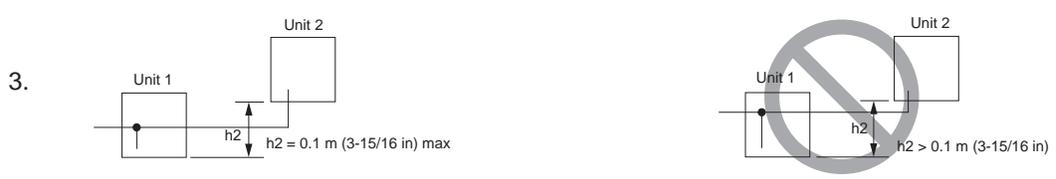
The NG example shows that oil accumulates into unit 1 while unit 2 is in operation, and unit 1 is stopped. Difference between unit and unit in height (h2) should be 0.1 m (3-15/16 in) or below.
