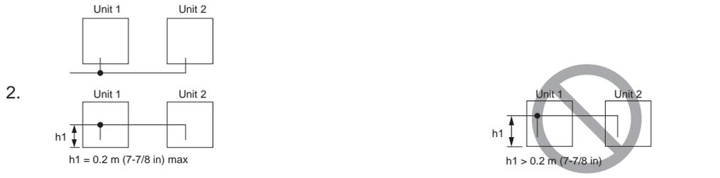
The NG example shows that oil accumulates into unit 1 while unit 2 is in operation, and unit 1 is stopped. Vertical pipe height (h1) should be 0.2 m (7-7/8 in) or below.
