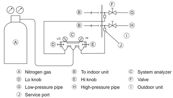
Observe the following restrictions when conducting an air tightness test to prevent negative effects on the refrigerating machine oil. Also, with nonazeotropic refrigerant (R410A), gas leakage causes the composition to change and affects performance. Therefore, perform the airtightness test cautiously.
