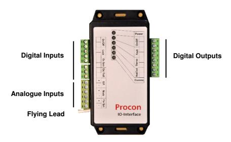
Connect the plug on the flying lead from the IO-INTERFACE to connector CN105 or CN92 on the associated air conditioner.
