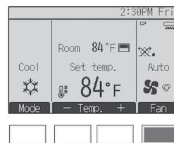
Press the [F4] button to go through the fan speeds in the following order.
