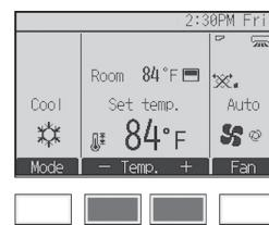
Press the [F2] button to decrease the set temperature, and press the [F3] button to increase.
