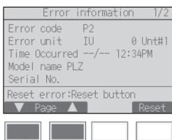
Error code, error unit, refrigerant address, unit model name, and serial number will appear.
