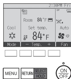
Press the HOLD button to enable/disable the HOLD function.
