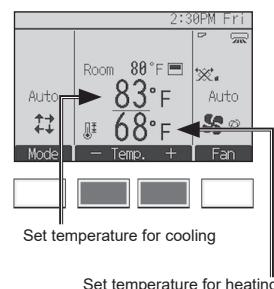
The current set temperatures will appear. Press the [F2] or [F3] button to display the Settings screen.
