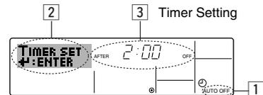
1. Be sure that you are at a standard control screen, and that the Auto Off timer indicator is visible in the display (at ①).
