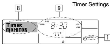
1. Be sure that the weekly timer indicator is visible on the screen (at ①).
