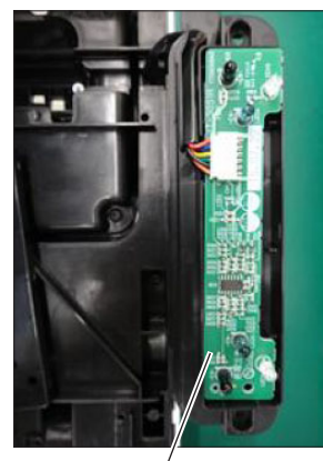
Light receiving circuit board (JT-30S1R)
