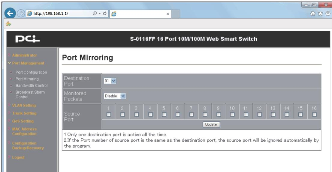
Configure the “Destination Port” setting for connecting the PC (Wireshark), and the “Source Port” setting for the monitoring target port. Multiple source ports can be selected. If “Tx & Rx” is selected for “Monitored Packets”, both sending and receiving packets can be captured.
