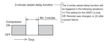
The unit has a function to keep the compressor from short-cycling when the amount of circulating water is low or when the load is light. After the compressor cycles off, it will not restart for 10 minutes.
