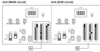
If the system is not started up for five minutes after the power is turned on (with the [EEEE] being displayed on the MAIN circuit), an error code [6500] or [7133] will appear on the SUB circuit. This error code will automatically light off once the system startup procedure is completed.
