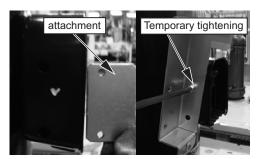
Hold the attachment and INJ pipe fixing plate against the terminal box, aligning the holes with the hole on the terminal box, and then temporarily screw in the top screw to hold them in place.
