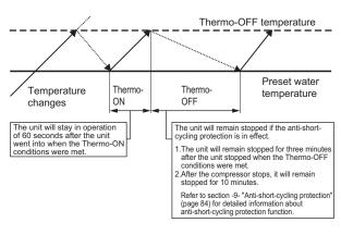
When the water temperature is controlled based on the inlet temperature, compressor frequency will be controlled as described in section -3- "Compressor frequency" (page 80). (Automatic operation according to the preset temperature)
