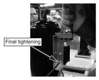
3. Tighten the fixing screw at the bottom.
