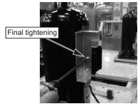
4. Tighten the fixing screw at the top.
