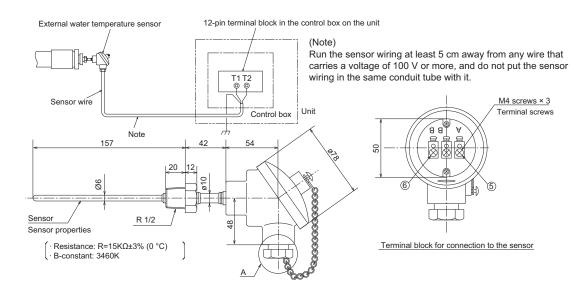
Connect the sensor wiring to terminals T1 and T2 of the 12-pin terminal block in the control box on the unit.
