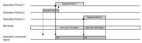
If two or more operation periods overlap, the settings for the period with a larger number will be ineffective. If Start time 1 and start time 3 are set to the same value, the setting for Start time 3 will be ineffective. Set the setting for Start time 3 to a time at least one minute after End time 1.
