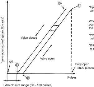
\*Upon power on, a 2260 pulse signal is sent to the LEV to determine the valve position and bring the valve to the position indicated by " A " in the diagram
