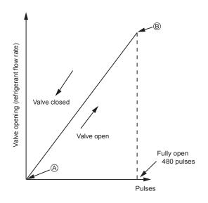
\*Upon power on, a 520 pulse signal is sent to the LEV to determine the valve position and bring the valve to the position indicated by " (A)" in the diagram. (Pulse signal is output for approximately 17 seconds.)
