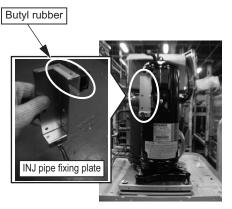
2. Press the butyl rubber on the fixing plate against the compressor shell.
