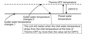
When the water temperature is controlled based on the external water temperature sensor reading (outlet water temperature), compressor frequency will be controlled in the way that the target water temperature will be maintained. If there is a sudden increase in water temperature and the unit did not stop at the preset temperature, the unit will stop when the temperature that equals "the preset temperature + the value set for DIFF2" is reached.
