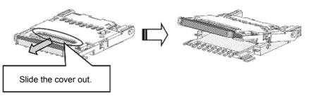
@Lift the cover up, and slide up the microSD card to remove it.
