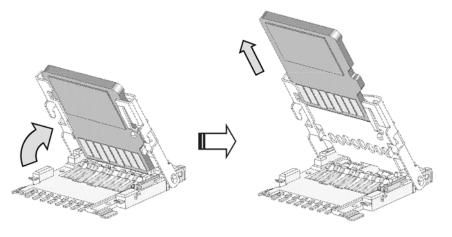
$\$ Close the cover, and slide the cover back in until the  $\Delta$  on the cover and the  $\Delta$  on the base are aligned to lock them in place.
