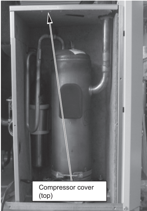
4. Remove the compressor cover (top).
