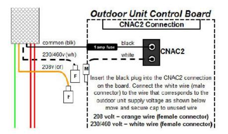
208/230 volt and also 460-volt outdoor units. On 208 volt units, the CNAC2 connector will provide 208 volts to the control transformer. On 230 volt units, the CNAC2 connector will provide 230 volts to the control transformer. The 460-volt units include a transformer that reduces the outdoor unit internal voltage to 230
