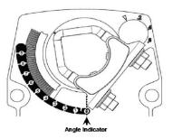
The factory setting for the mechanical stop is shown below at 85 degree hood angle.
