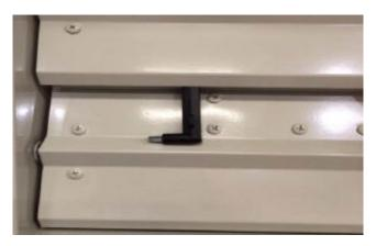
Step 7. Holding the blades against the handle re-tighten the (2) nuts on the damper shaft "U" clamp.
