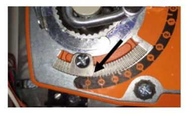
Step 3. Loosen the (2) nuts on the damper shaft "U" clamp.
