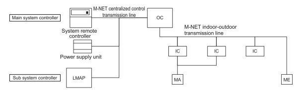
Figure 4-2. System configuration of system controller
