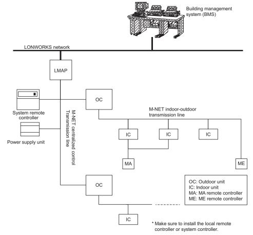
Figure 1-1. System configuration diagram (Example)
