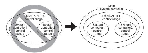
(2) In the case when the LM ADAPTER control range is covering the control range of the system controller partially, install the system controller so that it covers the entire control range of LM ADAPTER.
