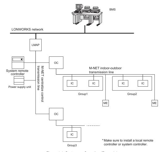
Figure 4-1. System configuration (Example)
