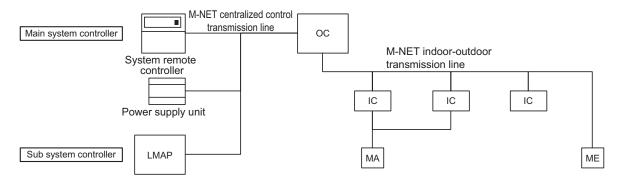
Figure 4-3. System configuration of local remote controller
