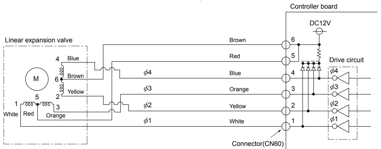
Note : Since the number of the connector at the controller board side and the relay connector are different, follow the color of the lead wire.
