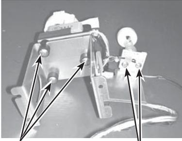
Drain pump fixing screw
