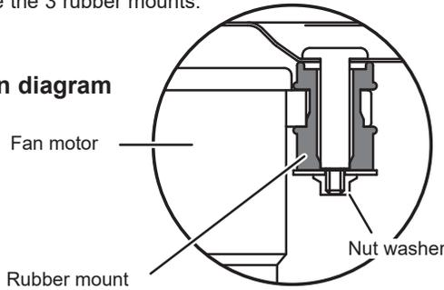
**Note:** When re-attaching the motor mount, make sure that the thicker end faces the motor shaft.
