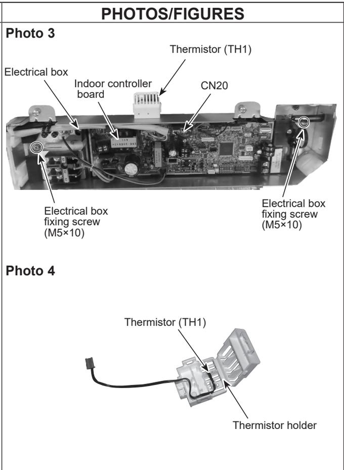
**5. Removing the indoor controller board (I.B)**
