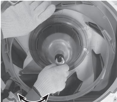
Turn this way to tighten. Turn this way to loosen.
