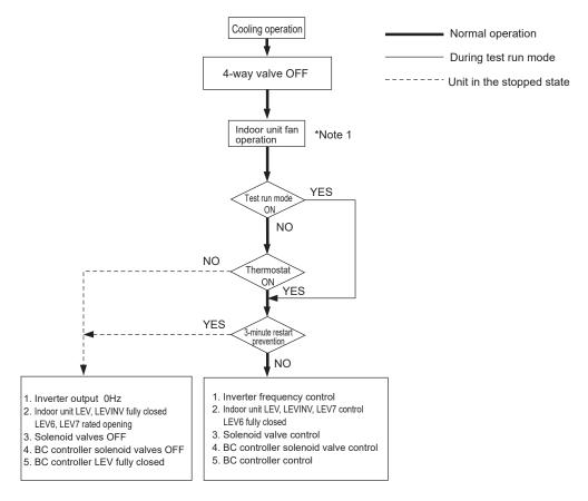
\*Note 1. The indoor fan operates at the set notch under cooling mode regardless of the ON/OFF state of the thermostat.
