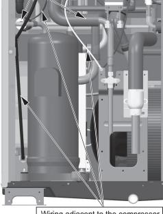
Wiring adjacent to the compressor
