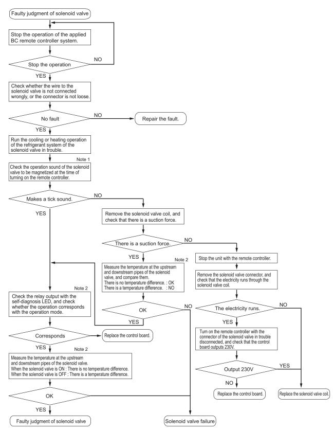
Check whether the BC board output signal corresponds with the solenoid valve operation correspond.
