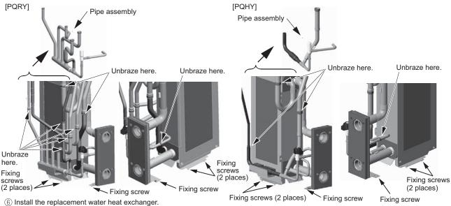
⑦ Reinstall the water heat exchanger fixing screws, solenoid valve block support, pipe support, pipe fixing plate and duct as they were.
