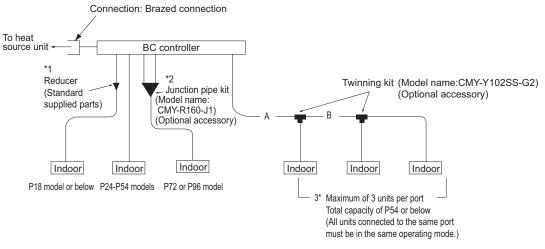
The ports of the BC controller accommodates the pipes on P24-P54 models of indoor units. To connect other types of indoor units, follow the procedure below.
