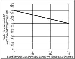
(2) System that requires more than 16 BC controller ports or with multiple BC controllers <Heat source unit P120 model or below>
