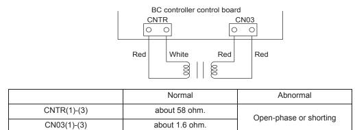
\* Before measuring the resistance, pull out the connector.
