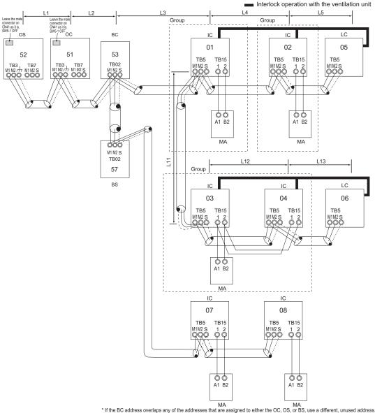
If the BC address overlaps any of the addresses that are assigned to either the OC, OS, or BS, use a different, unused add OC, OS, and BS addresses (lowest indoor unit address in the group plus +50) have higher priority than the BS address.
