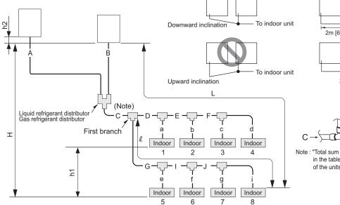
To indoor unit 2m [6ft] Joint pipe (gas pipe only) Trap (gas pipe only) To indoor unit 2m [6ft] Max. Joint pipe
