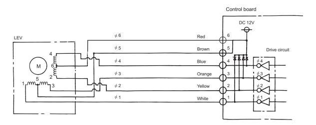
2) Pulse signal output and valve operation
