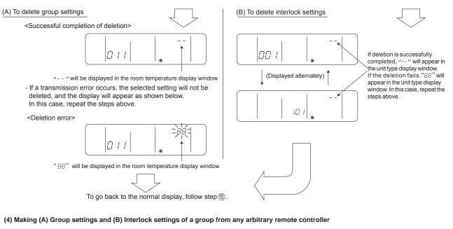
(A) Group settings and (B) Interlock settings of a group can be made from any arbitrary remote controller. Refer to "(B) Interlock Settings" under section 1 "Group Settings/Interlock Settings" for operation procedures. Set the address as shown below.
