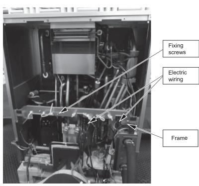
3. Remove the electrical wiring from the frame, unscrew the screws holding the check joint fixing plate, and remove the frame.
