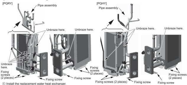
🕜 Reinstall the water heat exchanger fixing screws, solenoid valve block support, pipe support, pipe fixing plate and duct as they were.
