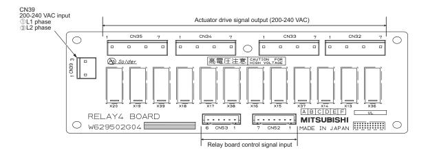
3. RELAY BOARD (RELAY 10 board)
