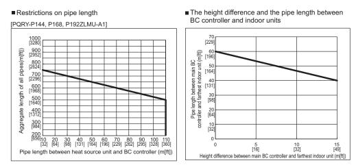
(2) System that requires more than 16 BC controller ports or with multiple BC controllers <Heat source unit P120 model or below>
