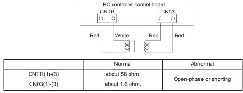
\* Before measuring the resistance, pull out the connector.
