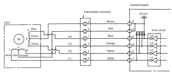
Note. The connector numbers on the intermediate connector and the connector on the control board differ. Check the color of the lead wire to judge the number.
