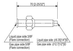
Note) Use the flare nut that is supplied with the BC controller.
