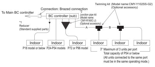
The ports of the BC controller accommodates the pipes on P24-P54 models of indoor units. To connect other types of indoor units, follow the procedure below.
