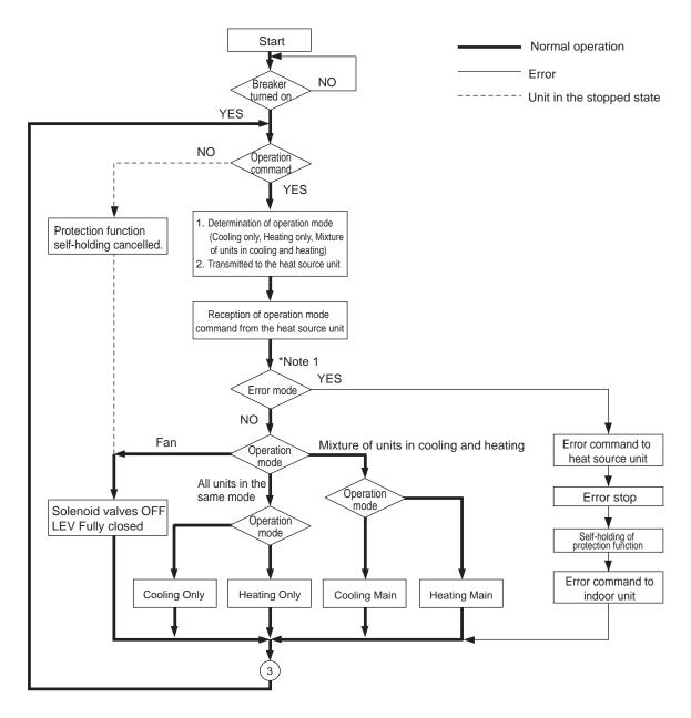
Note 1. The system may go into the error mode on either the indoor unit side or the BC controller or heat source unit side. If some of the indoor units are experiencing a problem, only those indoor units that are experiencing the problem will stop. If the BC controller or the heat source unit is experiencing a problem, all the connected units will stop. 2. Operations in each mode
