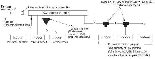
The ports of the BC controller accommodates the pipes on P24-P54 models of indoor units. To connect other types of indoor units, follow the procedure below.
