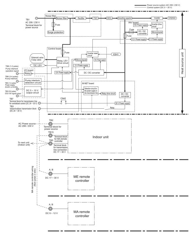
\* MA remote controllers and ME remote controllers cannot be used together. (Both the ME and MA remote controller can be connected to a system with a system controller.)
