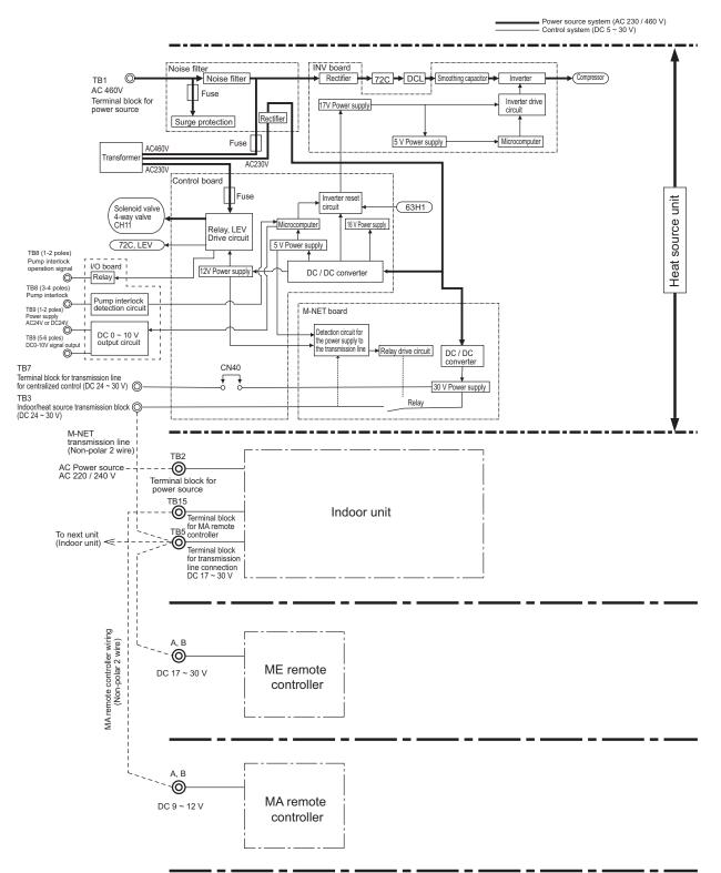
\* MA remote controllers and ME remote controllers cannot be used together.
