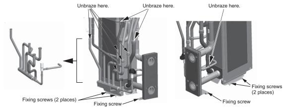
(6) Install the replacement water heat exchanger.
