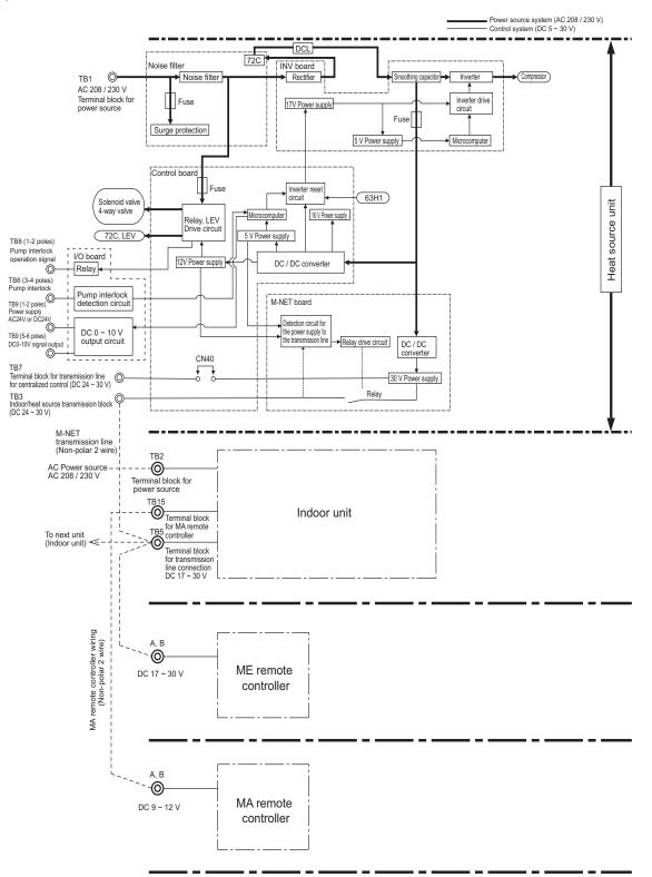
\* MA remote controllers and ME remote controllers cannot be used together.
