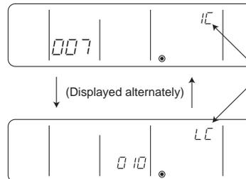
If registration is successfully completed, the two displays as shown on the left will appear alternately. If the registration fails, “BB” will blink on the display. (Indicates that the selected address does not have a corresponding unit.)
