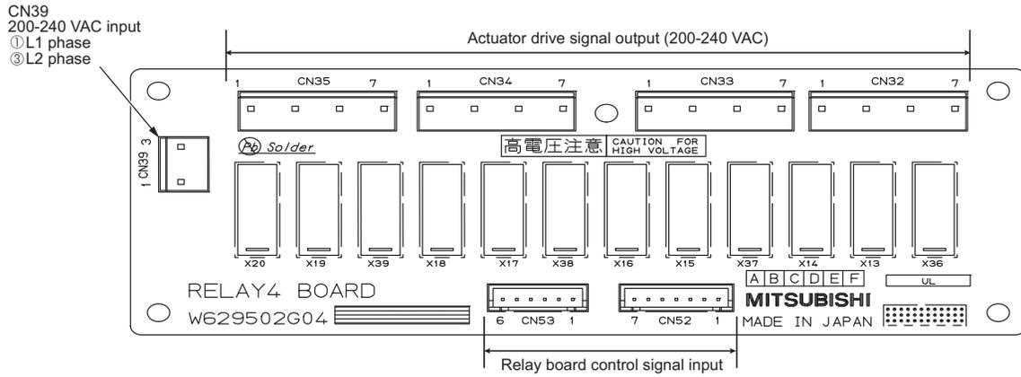
3. RELAY BOARD (RELAY 10 board)
