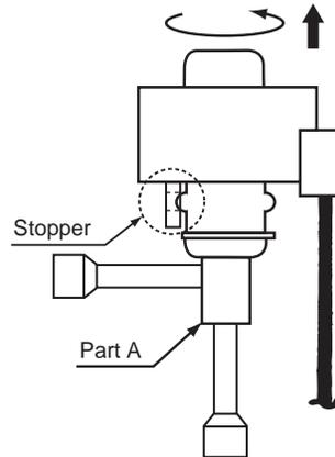
3) Installing the coil
