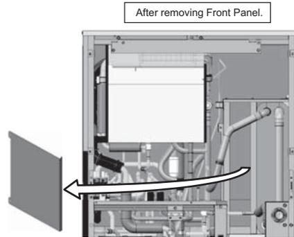
4) To move the Water Heat Exchanger and the Partition Plate
