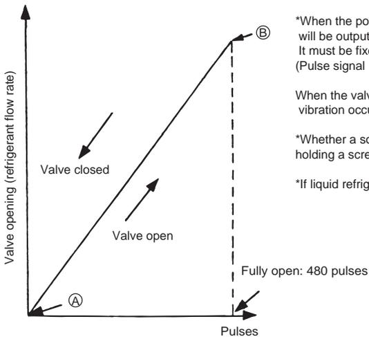
\*When the power is turned on, the valve closing signal of 520 pulses will be output from the indoor board to LEV to fix the valve position. It must be fixed at point (A)
