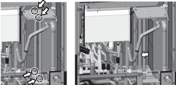
5) To remove the water heat exchanger
