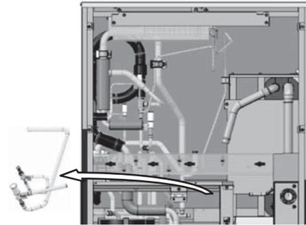
4) To remove the front panel of the Water Heat Exchanger and the side plate
