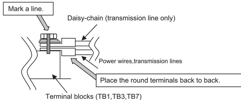
Poor contact caused by loose screws may result in overheating and fire.
