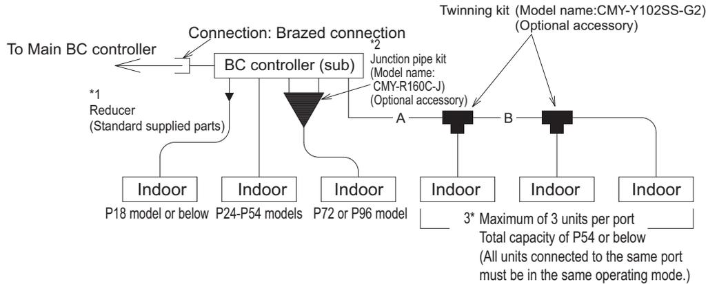
The ports of the BC controller accommodates the pipes on P24-P54 models of indoor units. To connect other types of indoor units, follow the procedure below.
