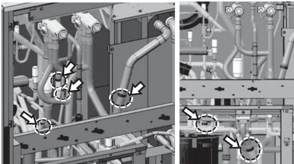
After removing 4-Way Valve Assy.
