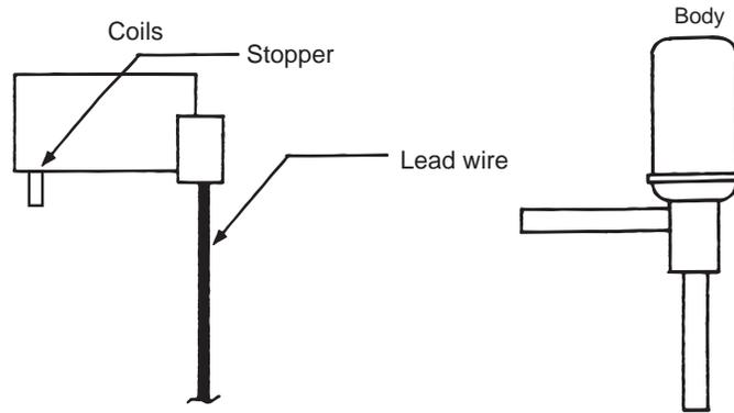
2) Removing the coils
