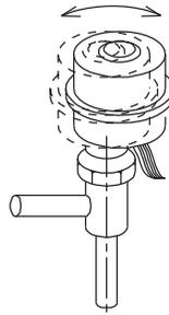
The motor may not be fixed with clamp because of the changing of the motor configuration. However, the fixing is not necessary due to the pipe fixing.
