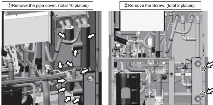
4) To remove the pipe from the Water Heat Exchanger
