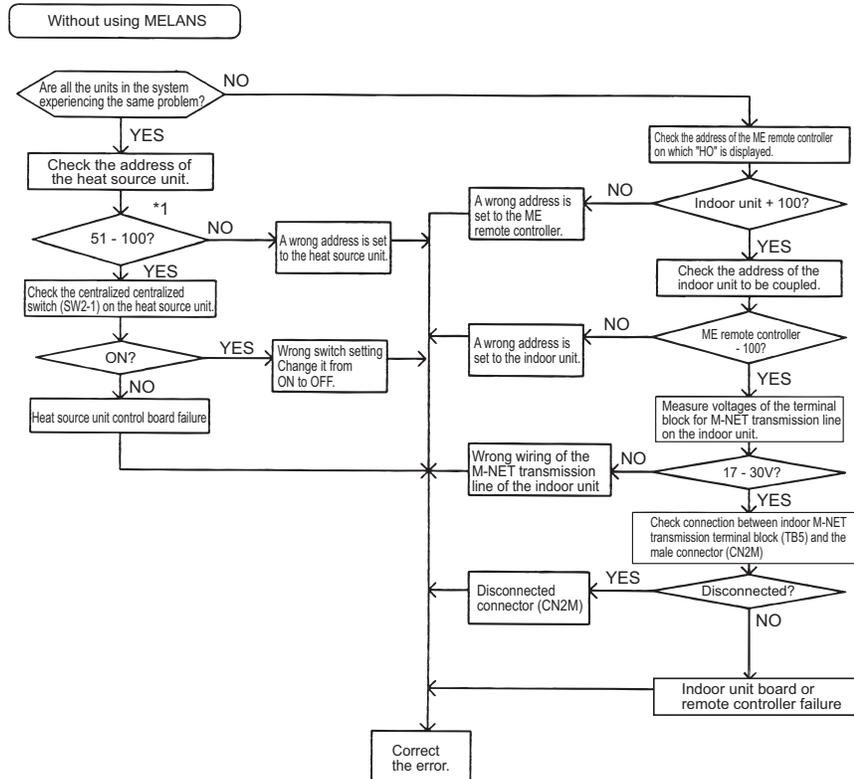
\*1. When the heat source unit address is set to 1 - 50, the address will be forcibly set to 100.
