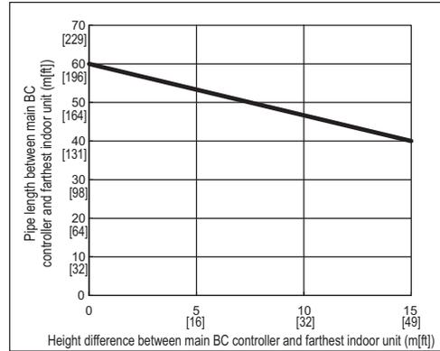
**(2) System that requires more than 16 BC controller ports or with multiple BC controllers <Heat source unit P120 model or below>**
