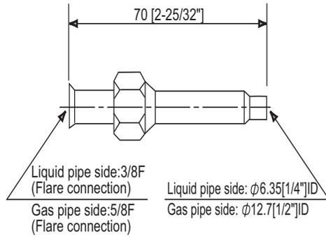
Note) Use the flare nut that is supplied with the BC controller.
