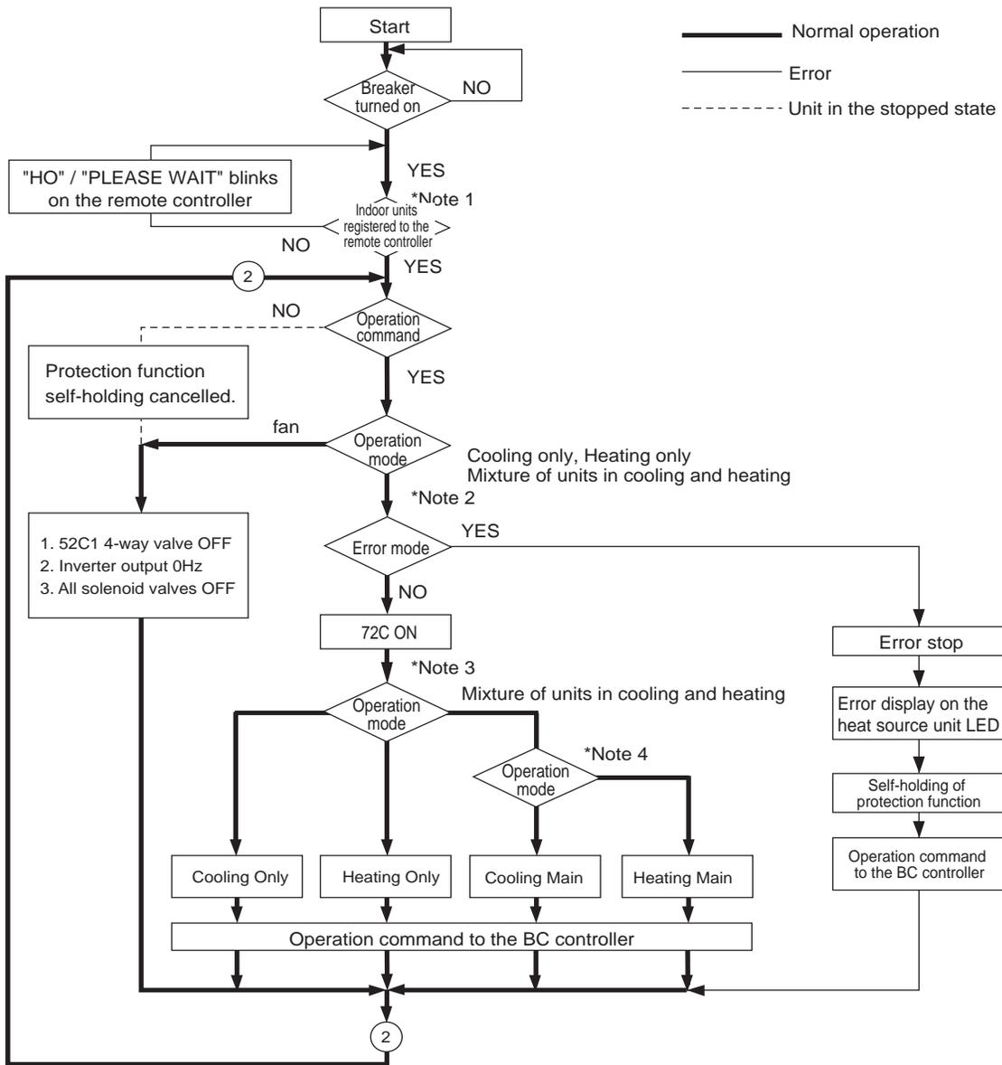
\*Note 1. For about 3 minutes after power on, search for the indoor unit address, for the remote controller address, and for the group information will start. During this, "HO"/ "PLEASE WAIT" blinks on the display of the remote controller. When the indoor unit to be controlled by the remote controller is missing, "HO"/ "PLEASE WAIT" keeps blinking on the display of the remote controller even after 3 or more minutes after power on.
