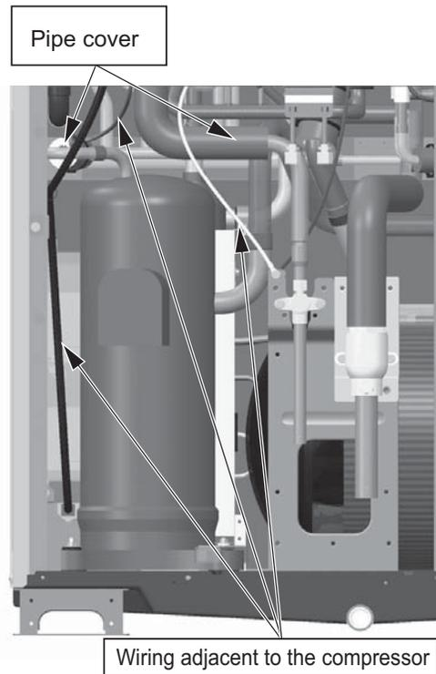
3. Remove the acoustic insulation material from the compressor. 4. First, move the nearby wiring and the pipe covers out of the way or protect them from the brazing flame; then debraise the pipe, and replace the compressor.
