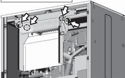
After removing Duct.
