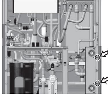
4) To remove the pipe from the Water Heat Exchanger
