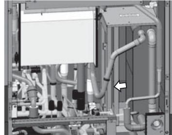
5) To remove the water heat exchanger
