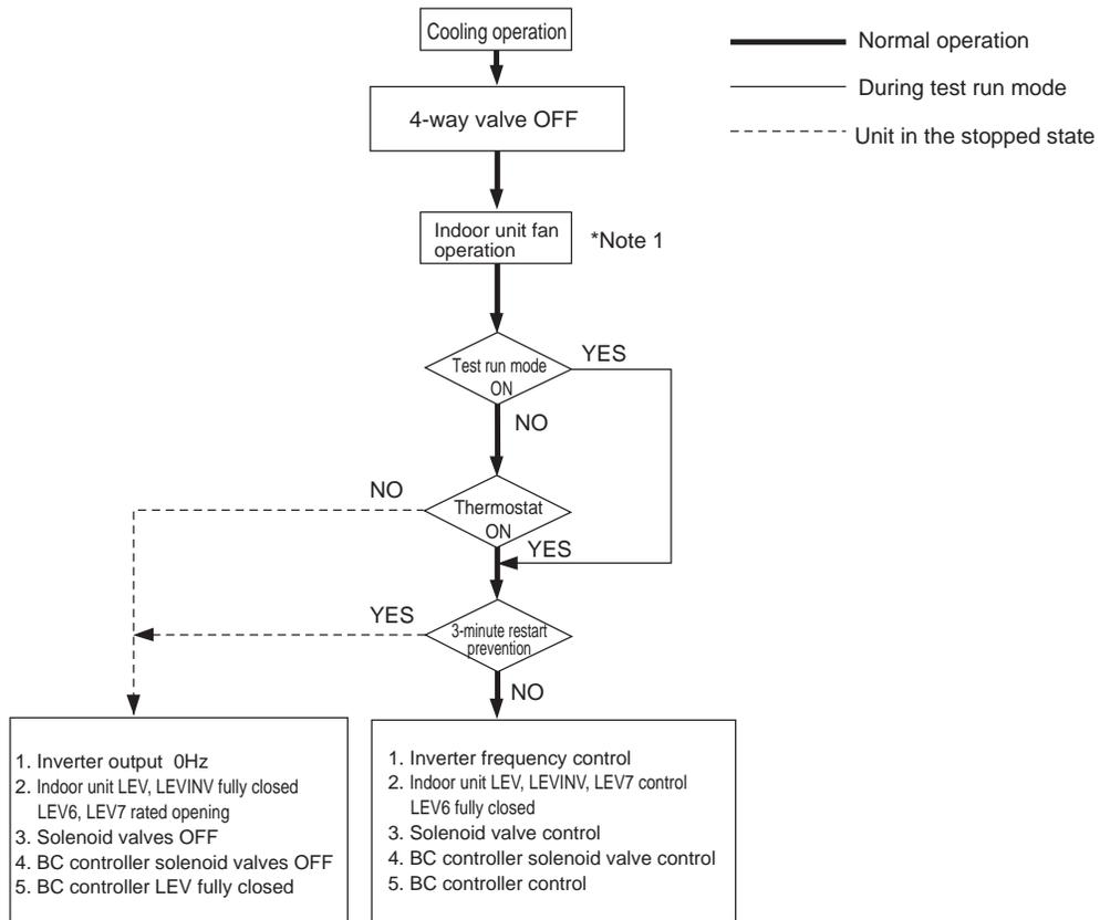
\*Note 1. The indoor fan operates at the set notch under cooling mode regardless of the ON/OFF state of the thermostat.
