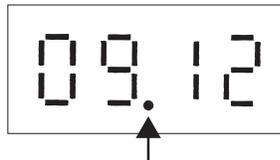
\* Disappears if the time data is deviated due to a power failure, or if a system controller that sets the time is not connected.
