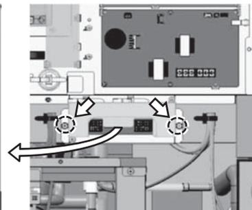
⑥ Remove the wire from cable strap on the Frame M.
