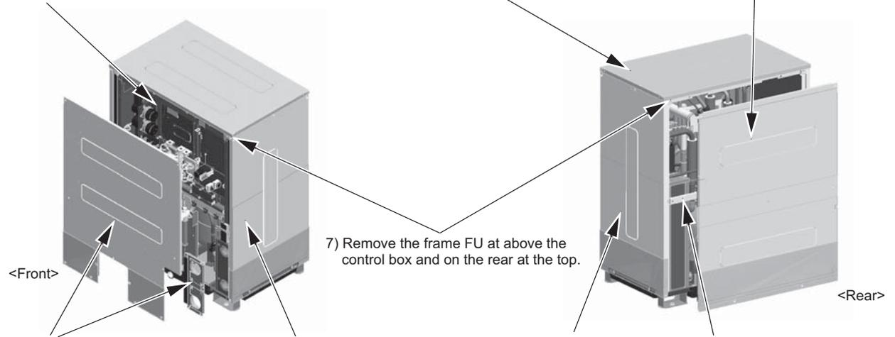
1) Remove the front (service) panel and the water pipe inlet/outlet panel.
