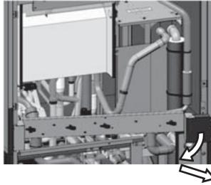
After removing Frame M.
