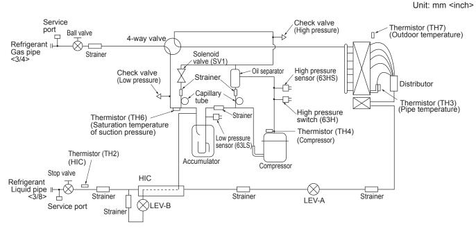
Capillary tube for oil separator :  $\phi$ 2.5 ×  $\phi$ 0.8 × L800 Capillary tube for solenoid valve :  $\phi$ 4.0 ×  $\phi$ 3.0 × L500
