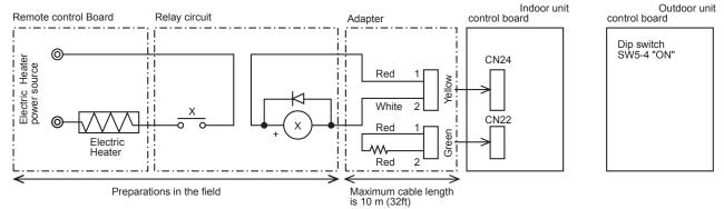
For relay X use the specifications given below operation coil
