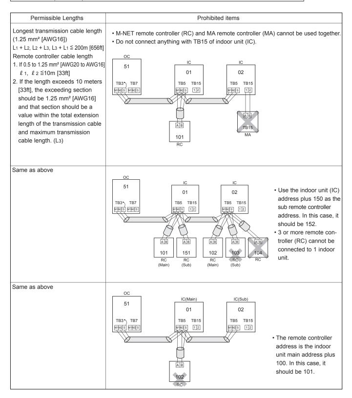
B. Example of a group operation system with 2 or more outdoor units and a M-NET remote controller. (Address settings are necessary.)
