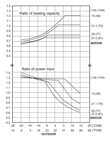
Figure 3 High heating performance curve
