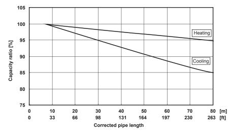
Figure 3 Capacity correction curve
