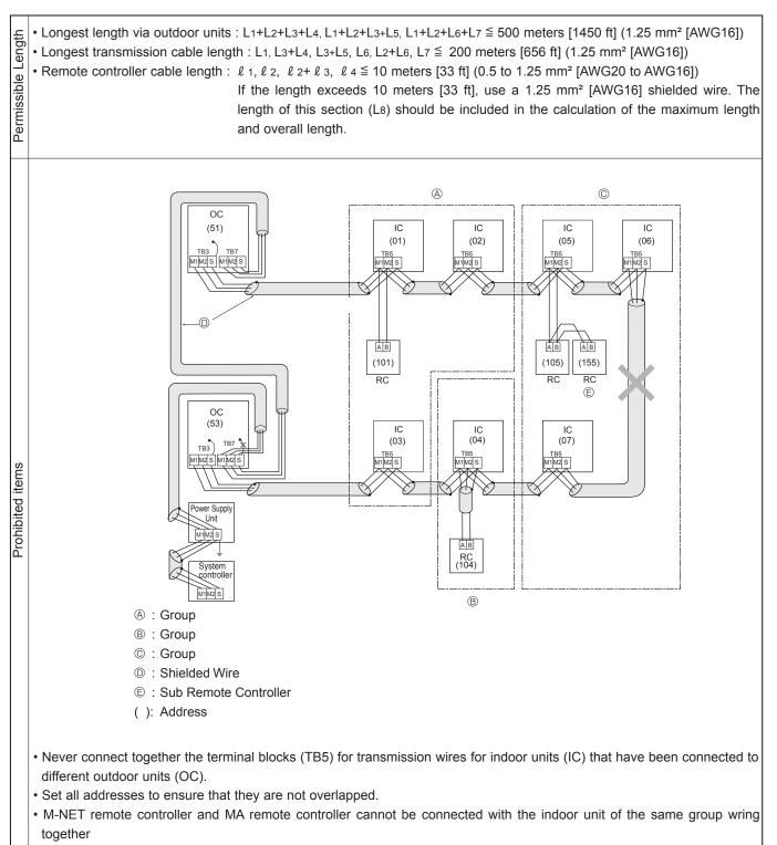
C. Example of a MA remote controller system (address setting is not necessary.) NOTE : In the case of same group operation, need to set the address that is only main indoor unit.
