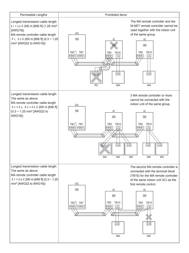
D. Example of a group operation with 2 or more outdoor units and a MA remote controller. (Address settings are necessary.)
