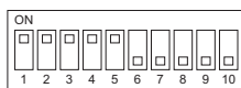
The figure at left shows that the switches 1 through 5 are set to ON and 6 through 10 are set to OFF.
