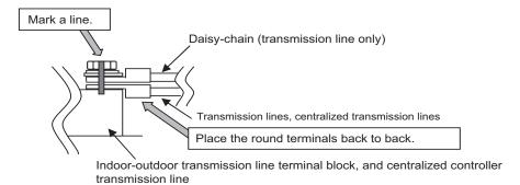
Poor contact caused by loose screws may result in overheating and fire. Continued use of the damaged circuit board may cause overheating and fire.
