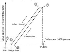
\*When the power is turned on, the valve closing signal of 2200 pulses will be output from the indoor board to LEV to fix the valve position. It must be fixed at point (A).
