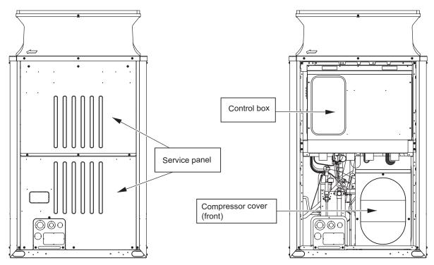
1. Remove both the top and bottom service panels (front panels).
