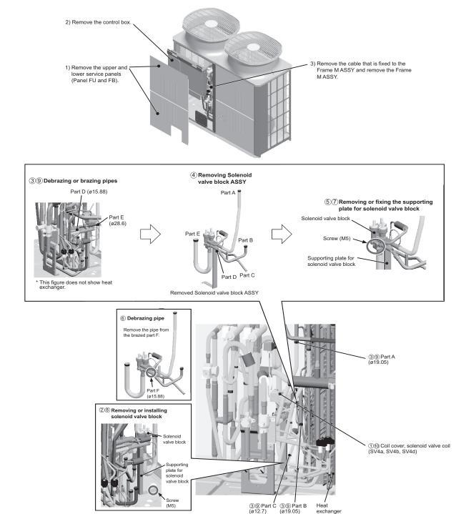
\* Refer to the next page for check valve (CV4a, CV6a, CV8a) replacement procedures.
