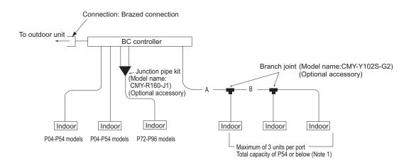
Note 1 Do not connect multiple indoor units to the same port when operating each of them in different mode (cooling, heating, stop, and thermo-off).
