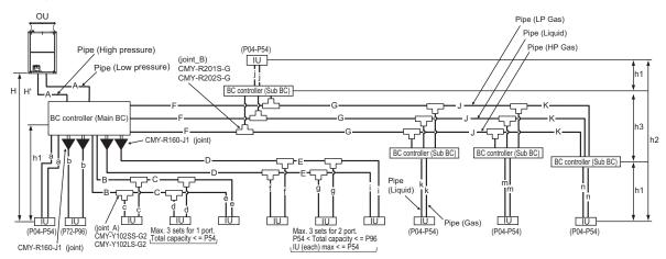
Fig. B Piping scheme OU: Outdoor unit. IU: Indoor unit
