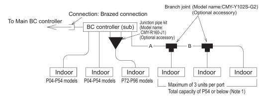
Note 1 Do not connect multiple indoor units to the same port when operating each of them in different mode (cooling, heating, stop, and thermo-off).
