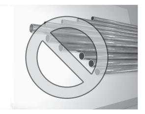
Both ends of the pipes should be sealed until just before brazing. Keep elbow pipes and T-joints in plastic bags.
