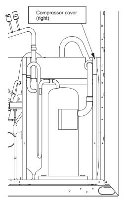
5. Remove the compressor wires and the compressor cover (right).
