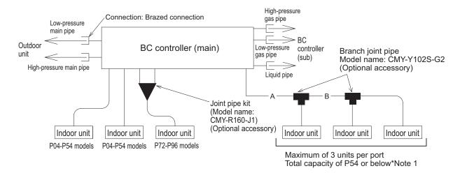
\*Note 1 Do not connect multiple indoor units to the same port when operating each of them in different mode (cooling, heating, stop, and thermo-off).
