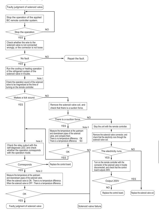
Check whether the BC board output signal corresponds with the solenoid valve operation correspond.
