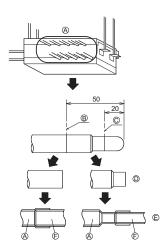
Be sure to have pipe expansion of indoor unit connecting port by cutting the piping at the cutting point which depends on the indoor unit capacity.
