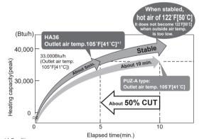
\*1 Condition Room temp. 70°F[21°C](D.B.) Outdoor temp. 35°F[1.7°C](D.B.) / 33°F[0.6°C](W.B.) : Hi notch
