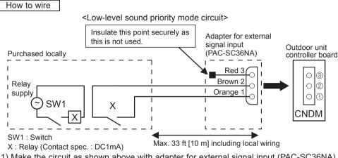
1) Make the circuit as shown above with adapter for external signal input (PAC-SC36NA).
