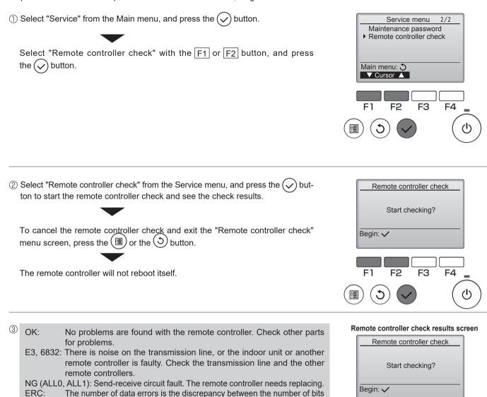
found, check the transmission line for external noise interference.
