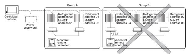
Note: In group B, M-NET address of the outdoor unit whose refrigerant address is "00" is not set to the minimum in the group. As "03" is right for this situation, the setting is wrong. Taking group A as a good sample, set the minimum M-NET address in the group for the outdoor unit whose refrigerant address is "00".
