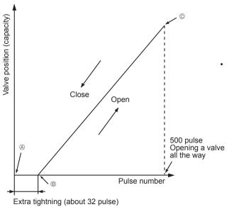
Opening a valve :  $8 \rightarrow 7 \rightarrow 6 \rightarrow 5 \rightarrow 4 \rightarrow 3 \rightarrow 2 \rightarrow 1 \rightarrow 8$ Closing a valve :  $1 \rightarrow 2 \rightarrow 3 \rightarrow 4 \rightarrow 5 \rightarrow 6 \rightarrow 7 \rightarrow 8 \rightarrow 1$ The output pulse shifts in above order.
