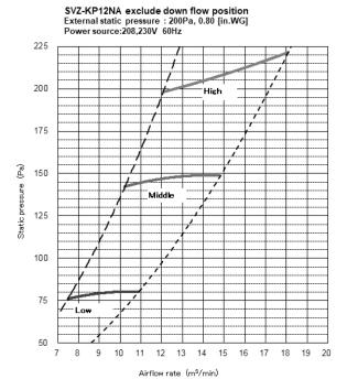
SVZ-KP12NA exclude down flow position External static pressure: 200Pa, 0.80 [in.WG] Power source: 208, 230V 60Hz
