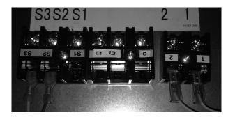
**Step. 10** Plug the connector from the Power Wiring Harness into CND. Connect the ground to the screw removed earlier and then connect the blue wire to "L1" and the red to "L2".
