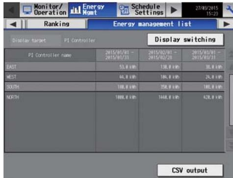
4. When the optional "Energy Management License Pack" is registered, up to four levels of peak-cut control can be set for the air conditioners and low-temperature devices to reduce the demand power. The history of average power and peak-cut control level can be confirmed on the energy management screen and output to a CSV file.
