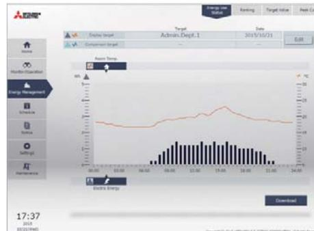
When the optional "Energy Management License Pack" is registered, up to four levels of peak-cut control can be set for the air conditioners to reduce the demand power.
