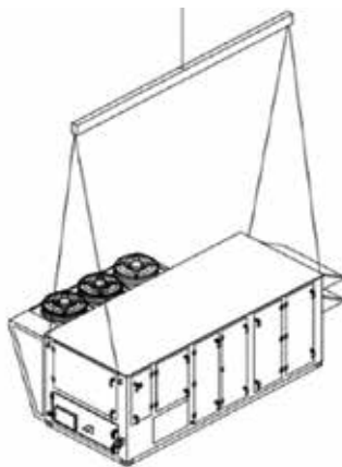
Lifting Details for MP 0, 1, 2, MPE 0, 1, 2, and MPC 1, 2
