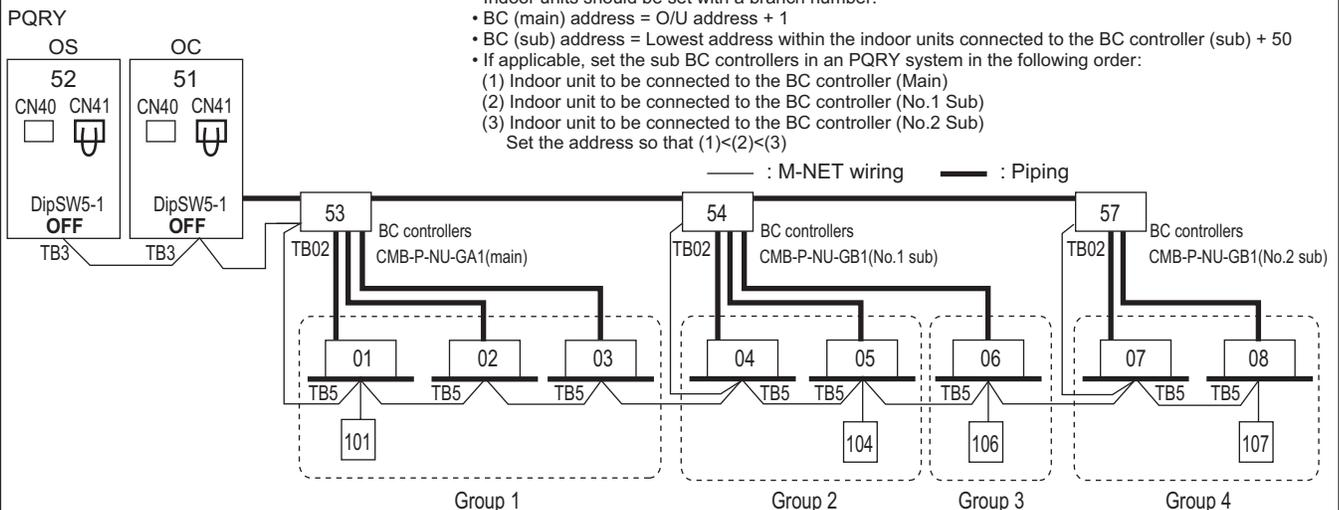
11-4-3-8. ME remote controller, Multi-refrigerant-system, No Power supply unit
