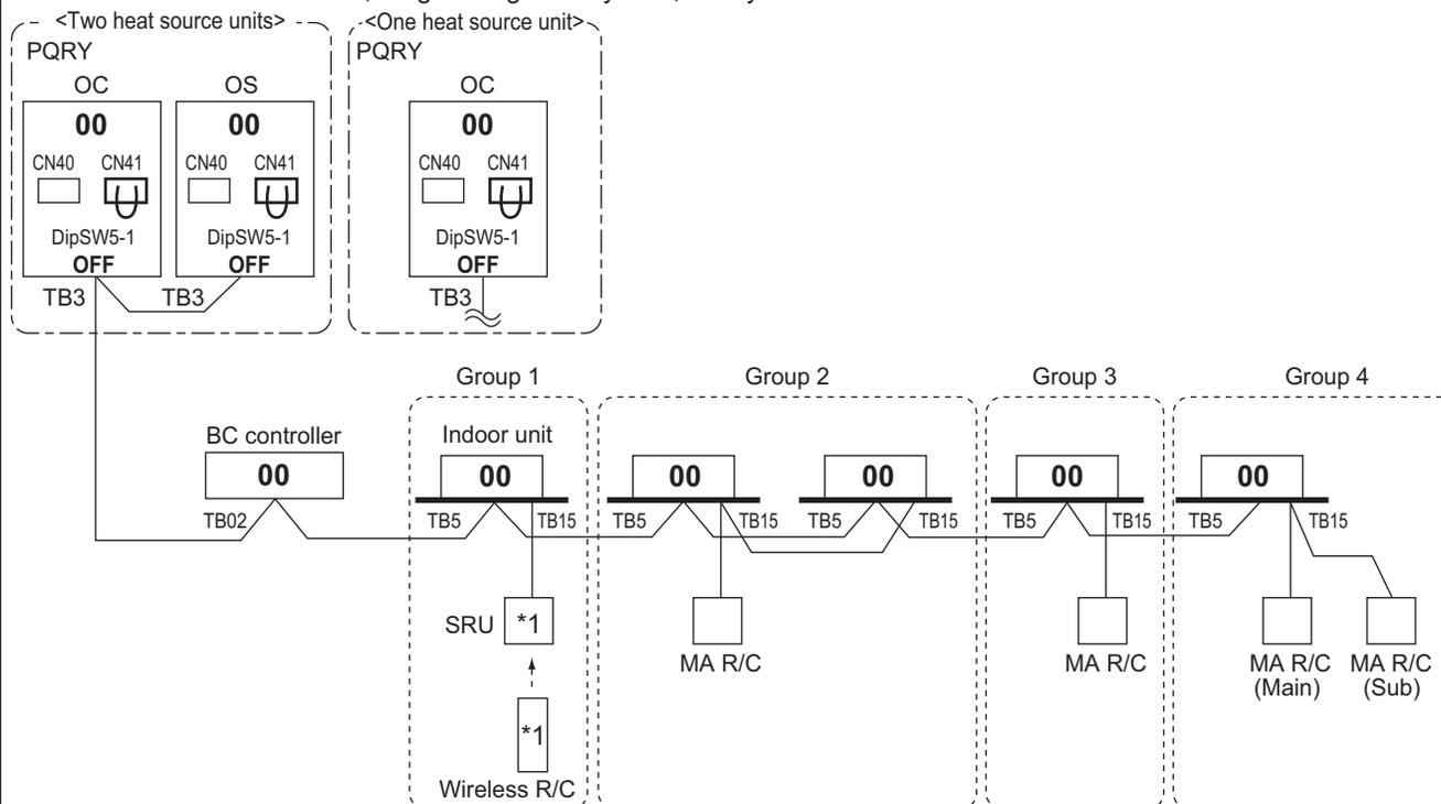
\*1 For Wireless R/C and Signal receiver unit (SRU), channel 1, 2 and 3 are selectable and should be set to same channel.
