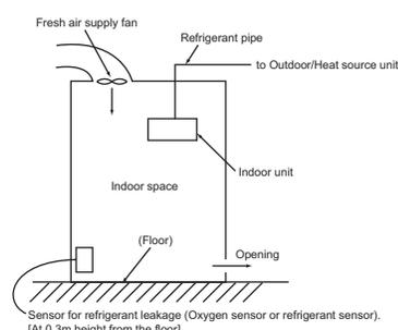
Fig. 1-3. Fresh air supply upon sensor action
