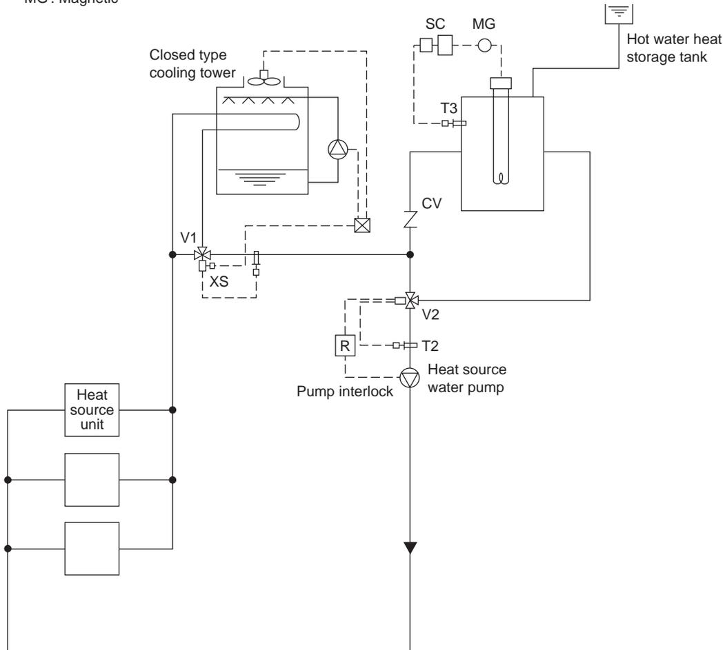
In the summer, as the circulation water temperature rises exceeding the set temperature of T1, the bypass port of V1 will open to lower the circulation water temperature. In the winter, if the circulation water temperature stays below 25°C [77°F], V2 will open/close by the command of T2 to keep the circulation water temperature constant.
