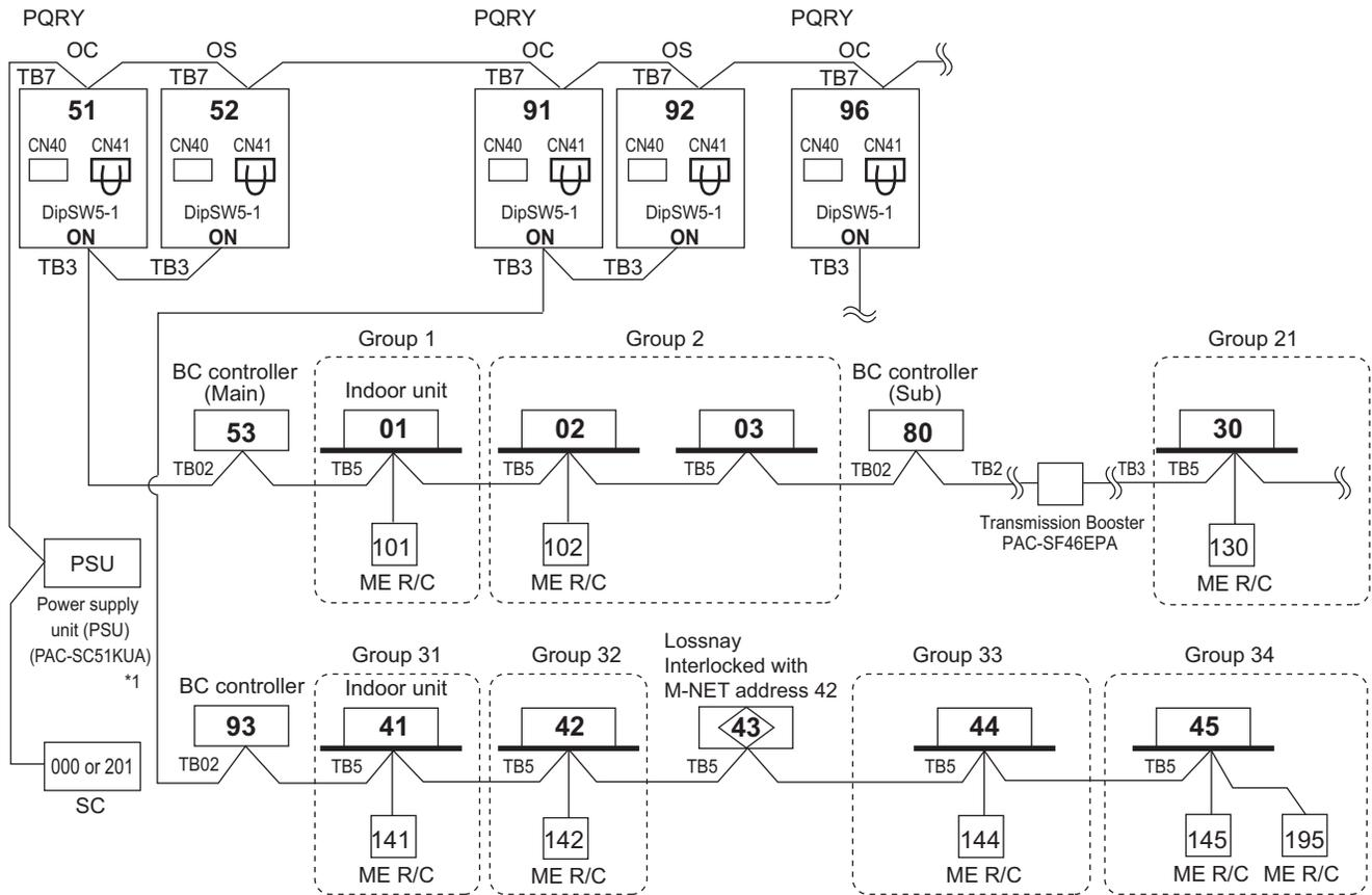
\*1 System controller should connect to TB7 at the Heat source unit and use power supply unit together in Multi-Refrigerant-System.
