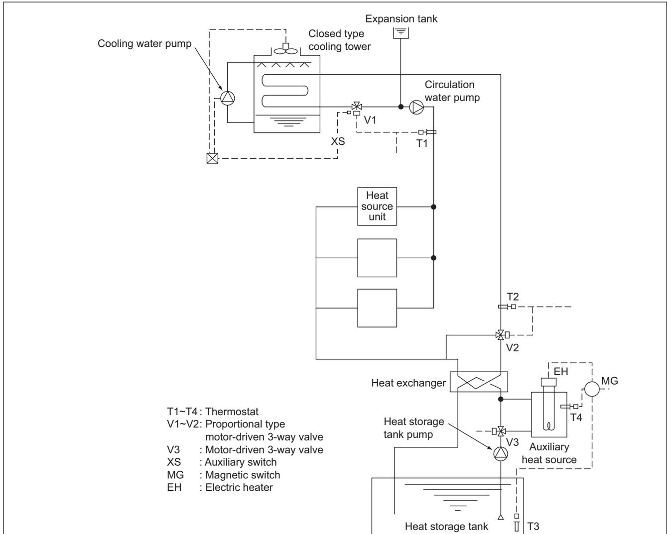
By detecting the circulation water temperature of the water heat source CITY MULTI system with T1 (around 32°C [90°F]) and T2 (around 20°C [68°F]), the temperature will be controlled by opening/closing V1 in the summer and V2 in the winter.
