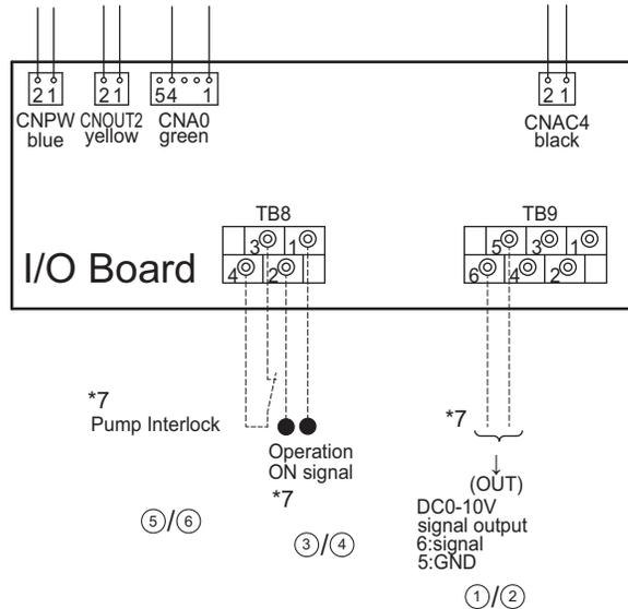
Figure d)-2 I/O board wiring diagram
