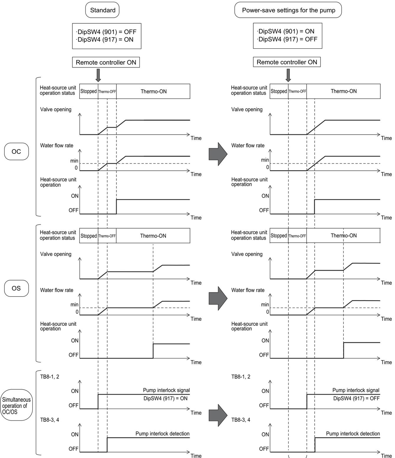
Circulating water stops when all heat-source units (OC/OS) are in the Thermo-OFF state.
