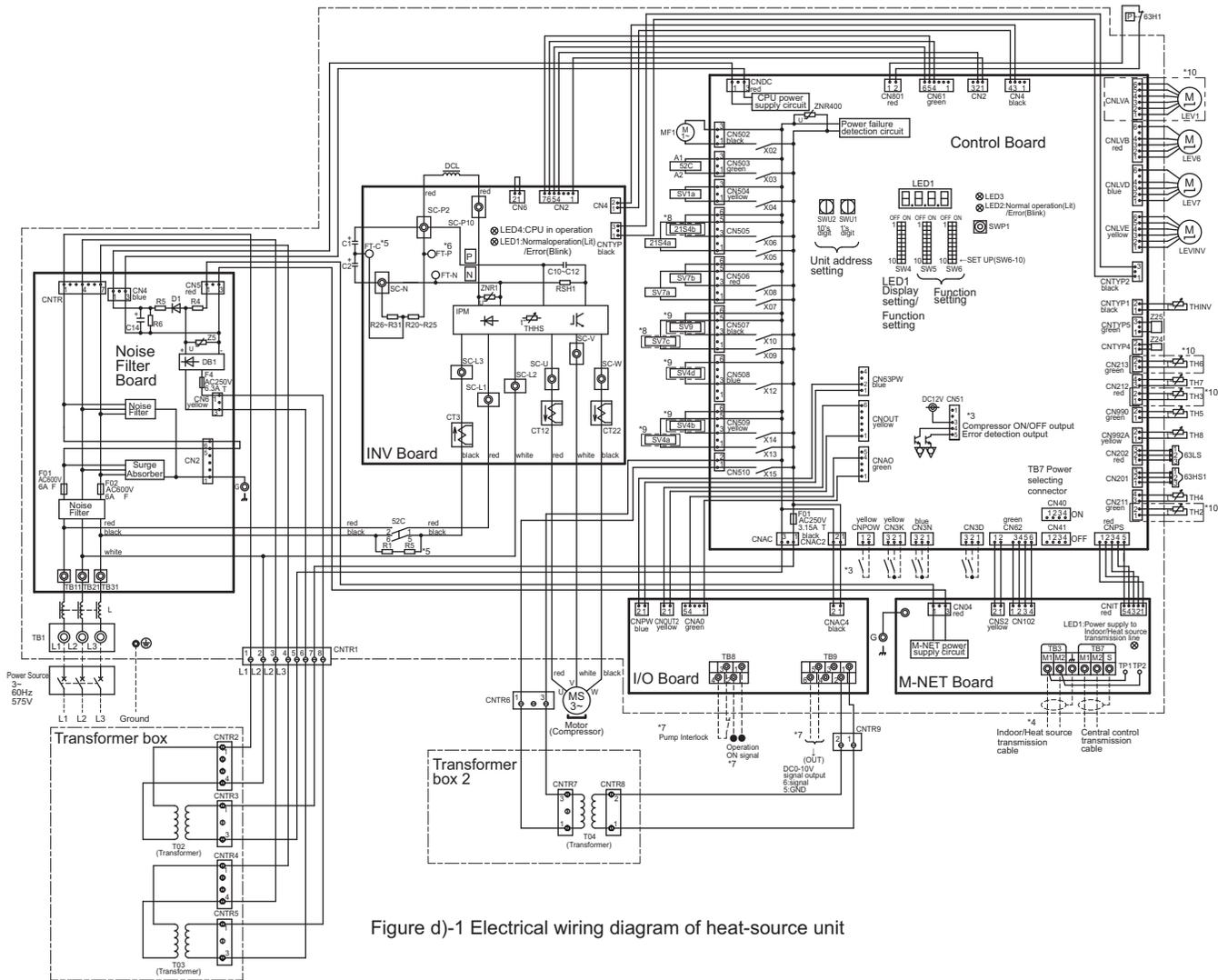
Figure d)-1 Electrical wiring diagram of heat-source unit
