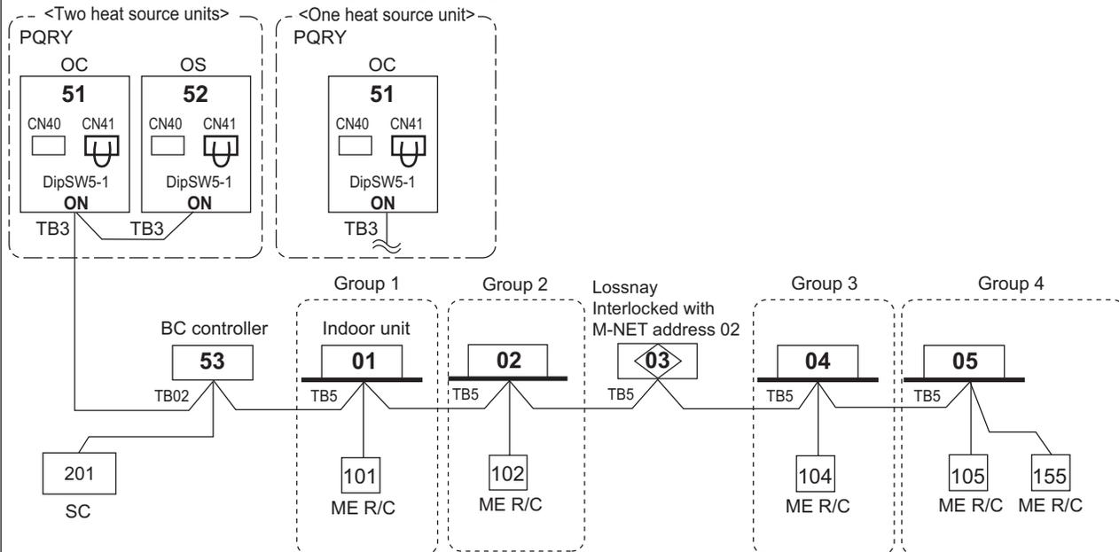
\*SC can be connected to TB3 side or TB7 side;
